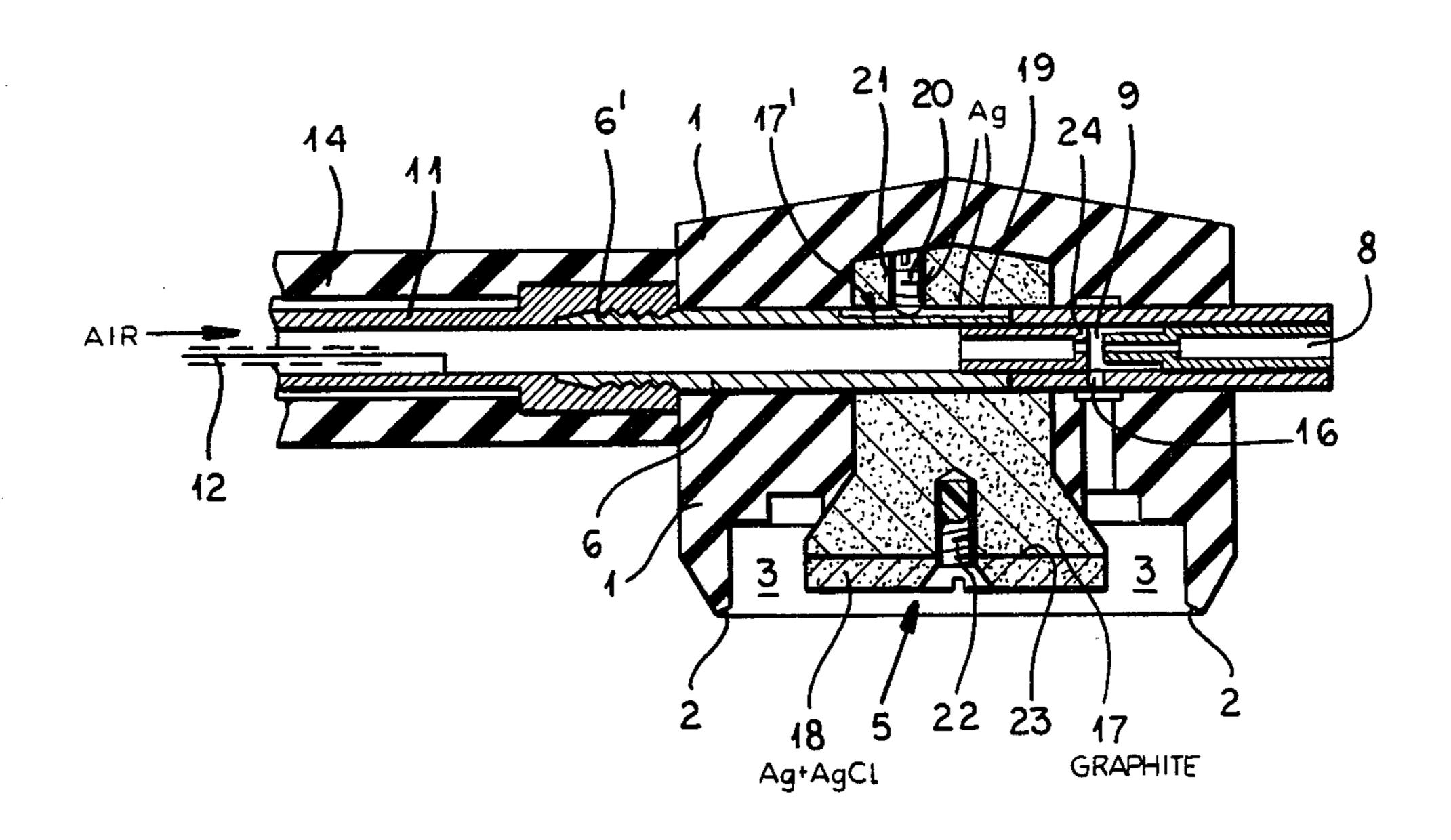
ELECTRODE STRUCTURE FOR ELECTRIC CONTACTOR
