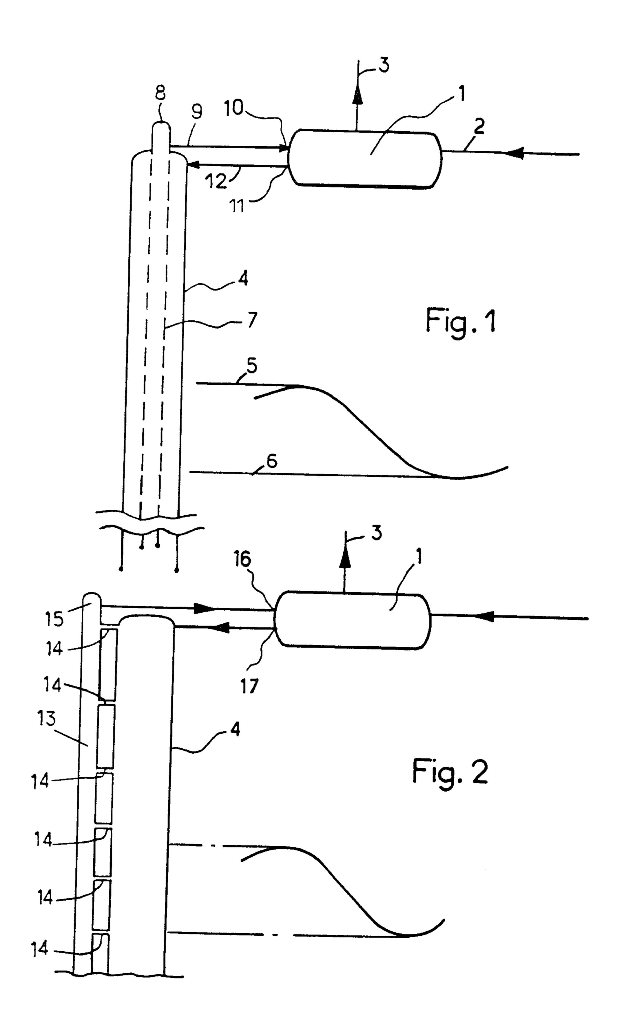
SAFETY SYSTEM FOR REMOVING ANY RISK OF CARRYING LIQUIDS TO THE NOSE OF THE FLARE OR TO THE VENT-HOLE DURING BURNING OR DISPERSION OF THE GASES ASSOCIATED WITH PRODUCTION
