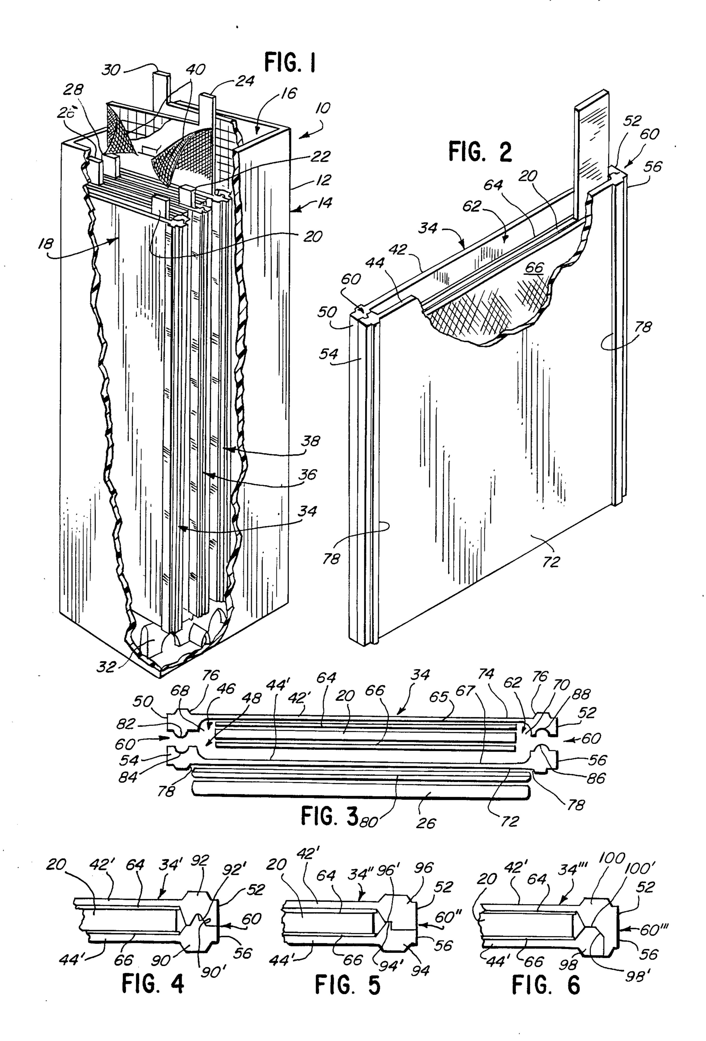
SEPARATOR PLATE FOR LEAD-ACID BATTERY
