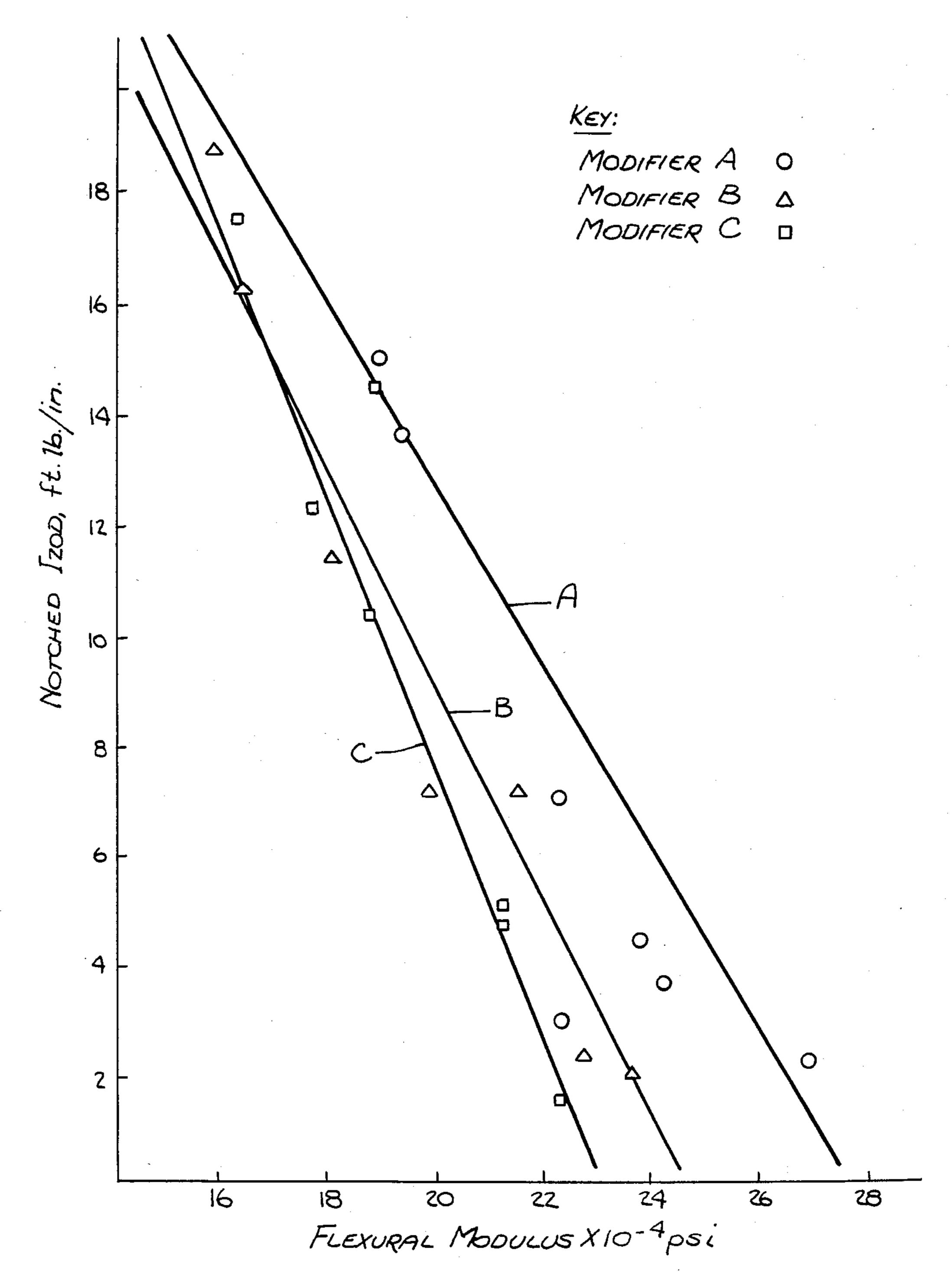
MODIFIER - NYLON 6/6 BLEND FLEXURAL MODULUS VS. NOTCHED IMPACT AT-40°F
