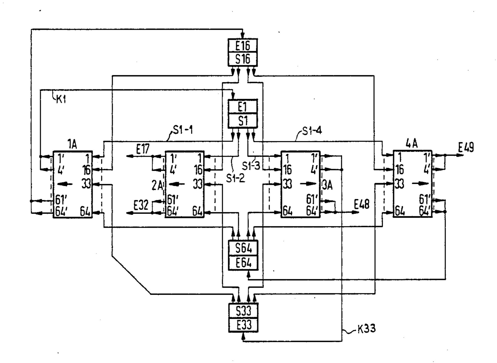
OPTICAL COUPLER NETWORK FOR COUPLING A PLURALITY OF SUBSCRIBER TRANSMITTERS TO A PLURALITY OF SUBSCRIBER RECEIVERS BY MEANS OF OPTICAL STAR COUPLERS
