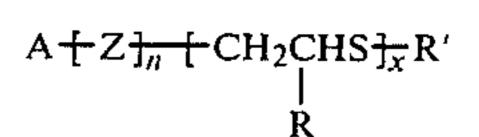
where A is the alkyl portion of the initiator, Z is a repeating monomeric unit of a monomer susceptible to anionic polymerization or mixtures of said monomers, n is a positive integer from 3 to 1500, R is hydrogen, C<sub>1</sub>-C<sub>10</sub> alkyl, or phenyl, x is a positive integer of at least 1, and R' is a radical formed by removal of halogen from a halogenated compound containing a polymerizable moiety.
