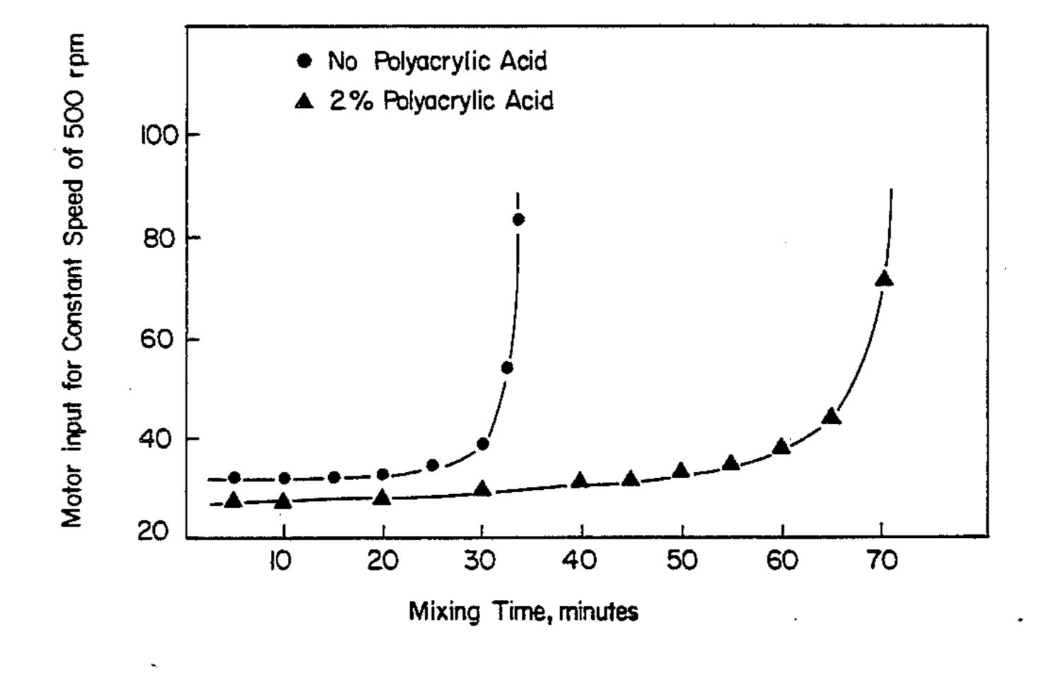
Effect of Polyacrylic Acid on Low Shear Thickening Time of Well Control Fluid
