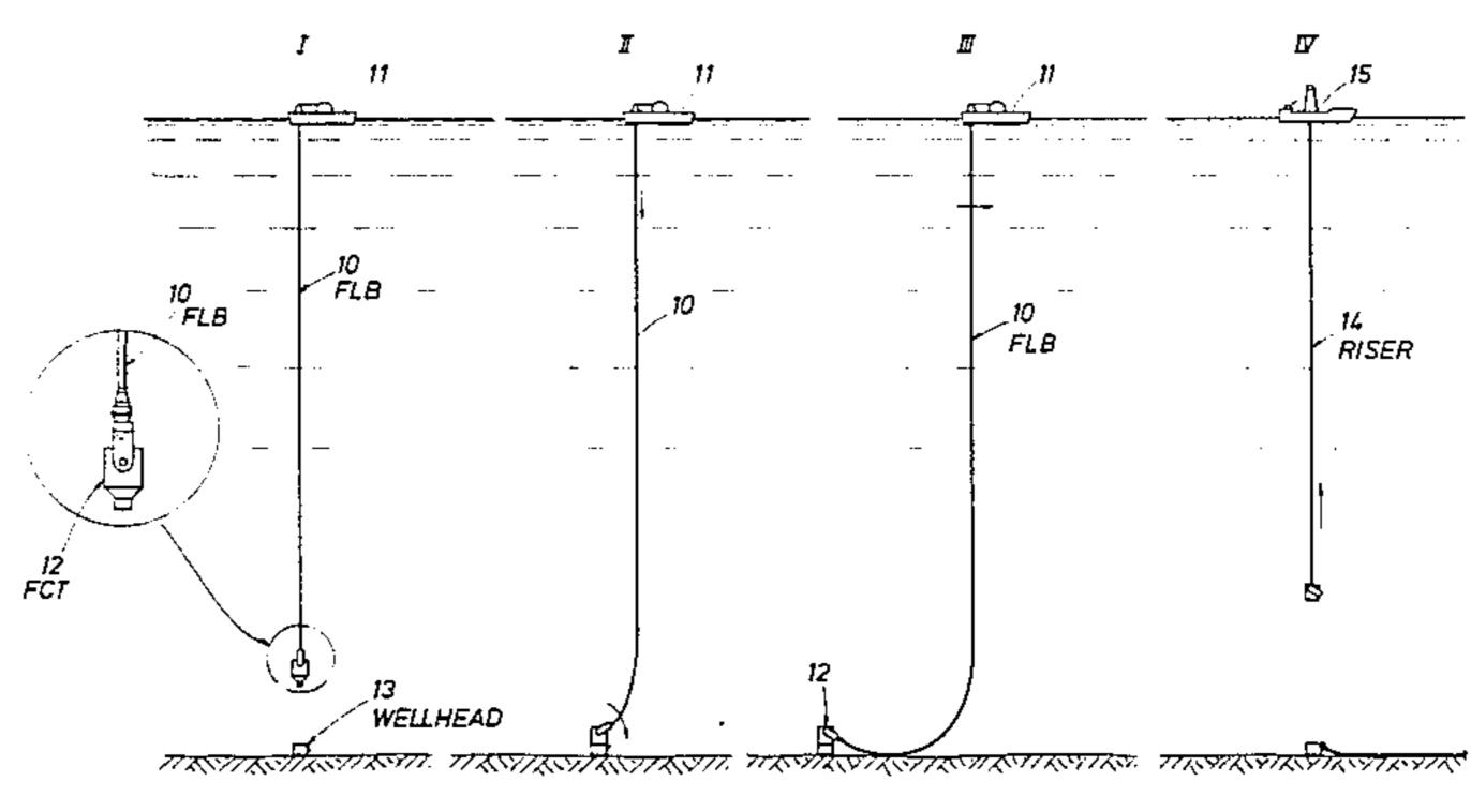
1. LAND FCT ONTO WELLHEAD 2 BEGIN HINGEOVER AND PIPELAY
