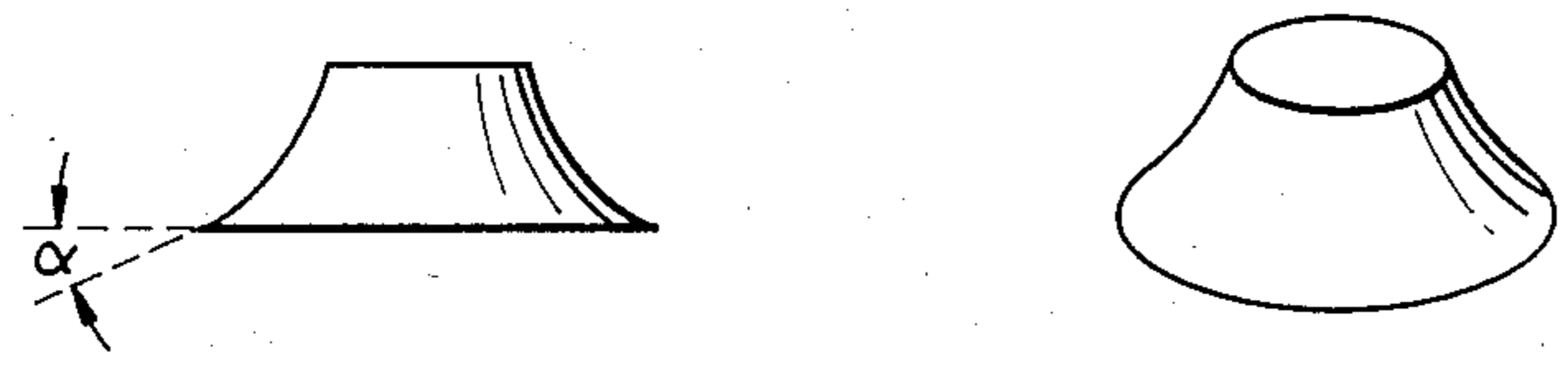
NO.5 Curved Taper Pin ( \alpha = 65^\circ )
