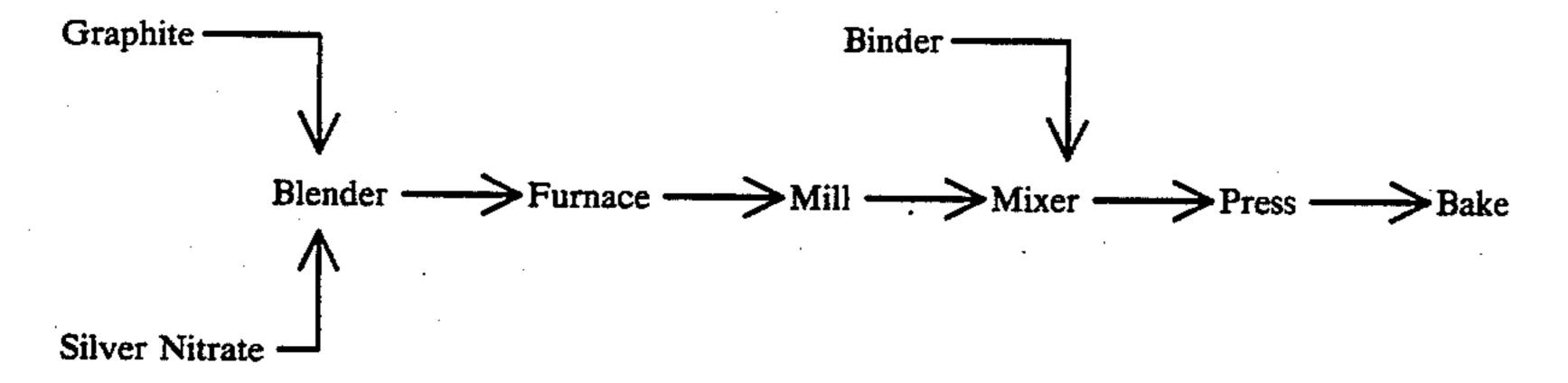
In accordance with this invention, graphite and silver nitrate are blended together and heated to an elevated temperature of 600° to 800° C. or to where the silver 55 nitrate is converted to metallic silver. The mixture of silver-graphite is milled and combined with a binder and a solvent in a mixer. This blend is milled and molded into desired shapes and baked. The raw materials can be mixed in any proportions to obtain the desired 60 product of silver in the product.
