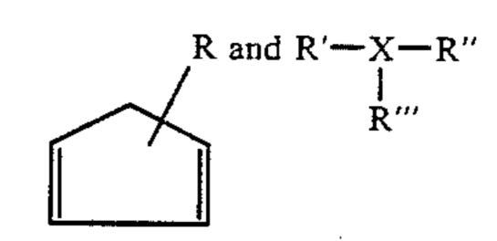
wherein R, R', R" and R" are radicals independently selected from the group consisting of hydrogen, C<sub>1</sub> to C<sub>20</sub> alkyl, C<sub>3</sub> to C<sub>20</sub> cycloalkyl, C<sub>6</sub> to C<sub>20</sub> aryl, C<sub>7</sub> to C<sub>20</sub> aralkyl and alkaryl, and X is selected from the group consisting of N, P, As and Sb, a is a positive integer ranging from 1 to 5 and b is an integer ranging from 0 to 4, with the proviso that the sum of a and b is 5 or less.
