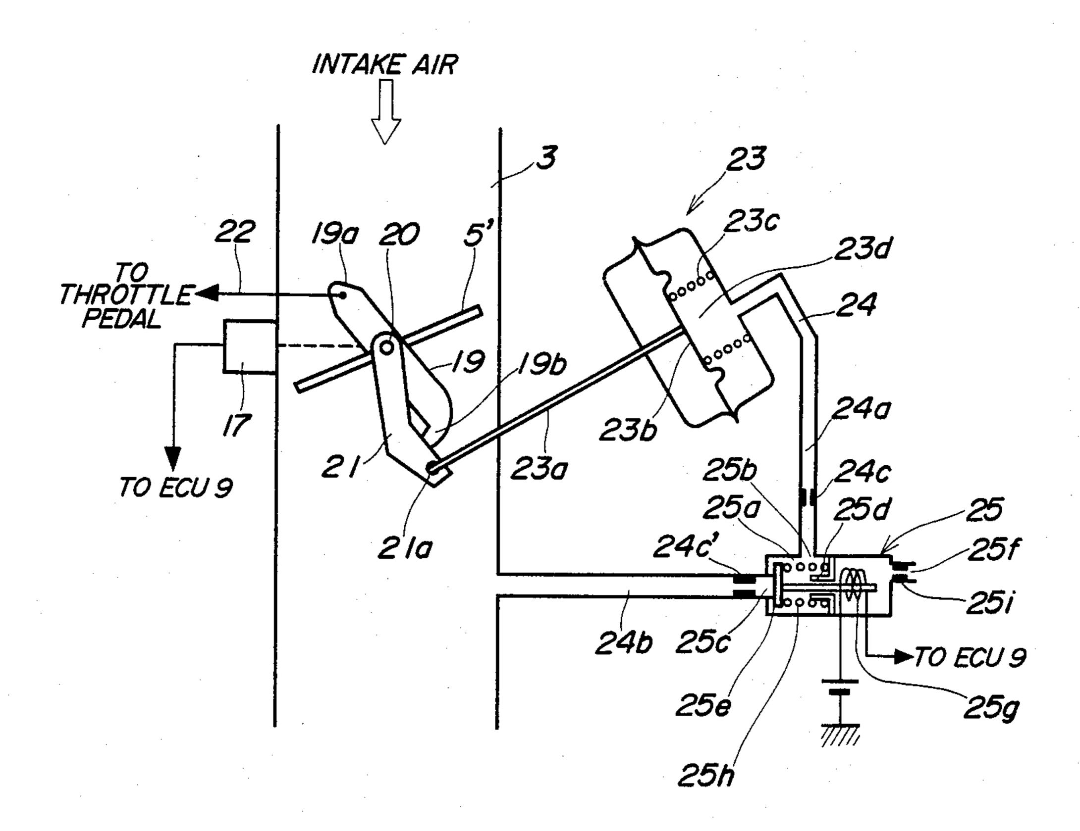
IDLING SPEED FEEDBACK CONTROL METHOD HAVING FAIL-SAFE FUNCTION FOR ABNORMALITIES IN FUNCTIONING OF CRANK ANGLE POSITION-DETECTING SYSTEM OF AN INTERNAL COMBUSTION ENGINE
