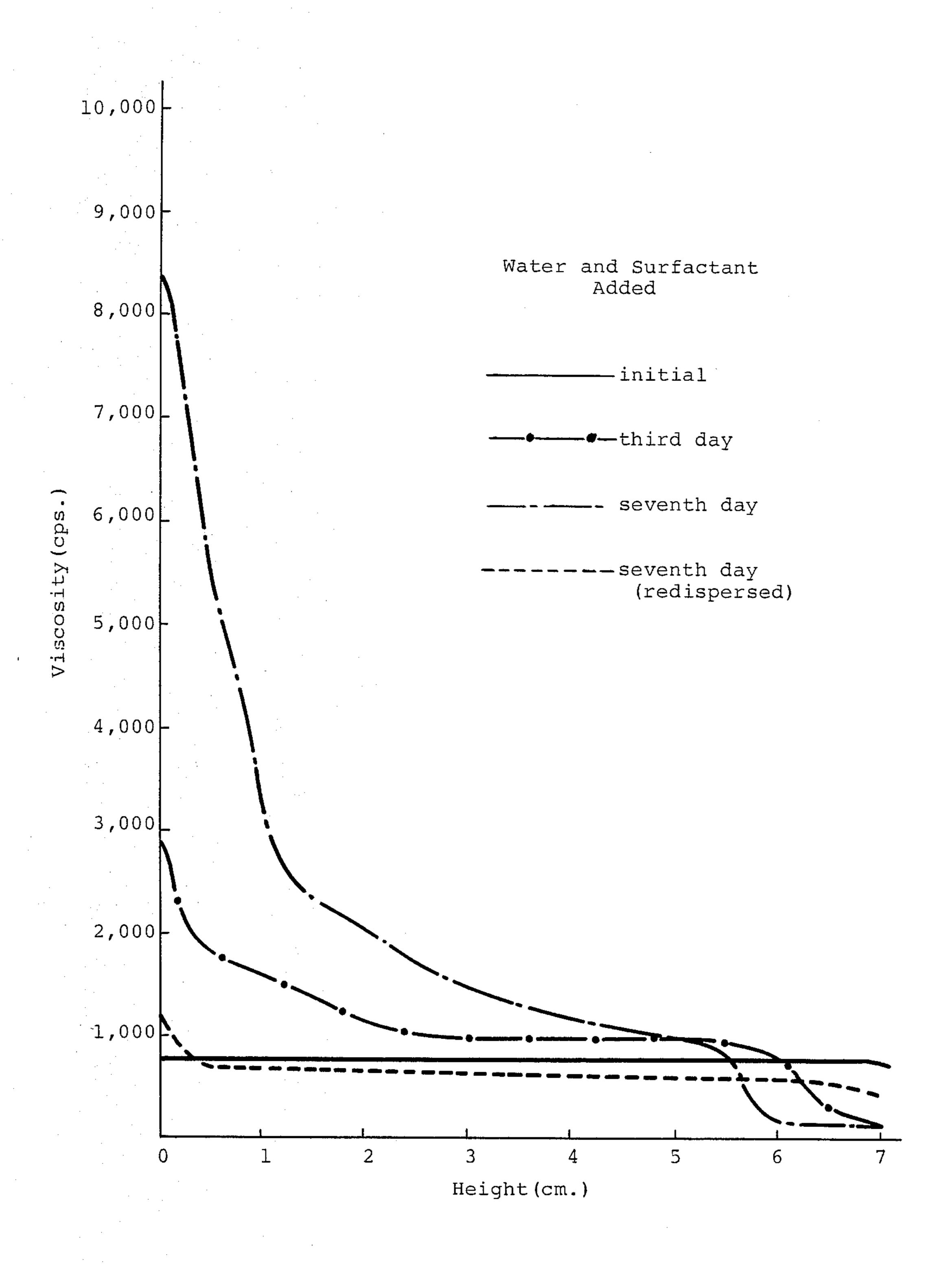
FIG. 3 SEDIMENTATION CHARACTERISTICS OF OF 30% PULVERIZED COAL IN #6 FUEL OIL
