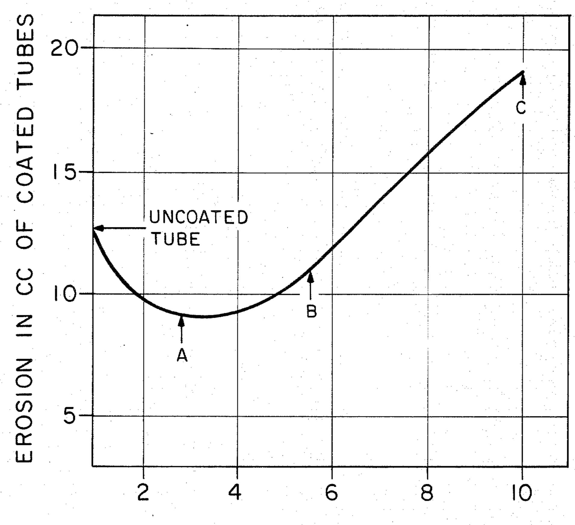
COLLOIDAL SILICA CONTENT OF COATING, %
