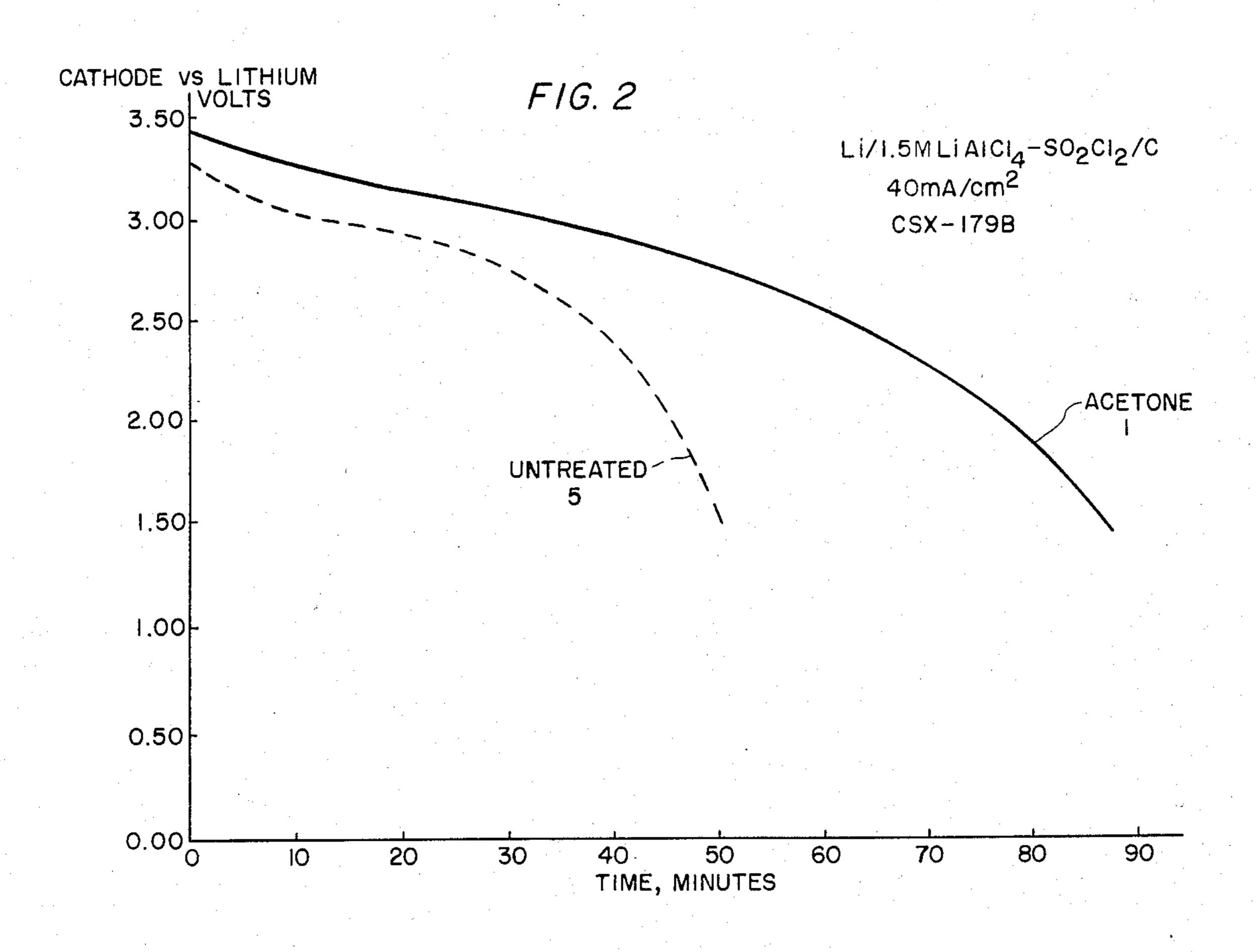
METHOD OF PRETREATING CARBON BLACK POWDER TO IMPROVE CATHODE PERFORMANCE AND LITHIUM SULFURYL CHLORIDE CELL INCLUDING THE PRETREATED CARBON BLACK POWDER
