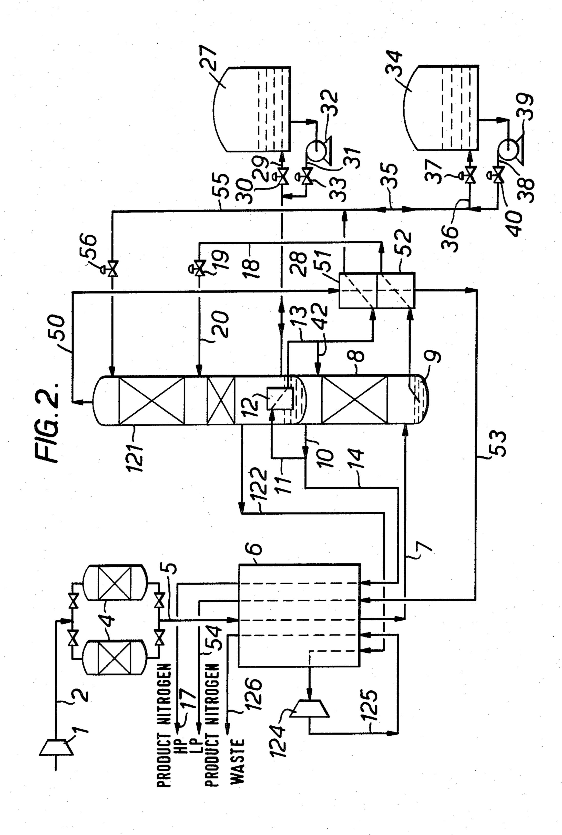
PLANT FOR PRODUCING GASEOUS NITROGEN
