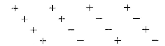
It should be noted that the fourth column has the same sign (+) as the fifth column. Thus, the distribution of these electrodes can be differently organized to make the columns having the same sign coincide, which makes it possible to reduce their number. For example, 40 the following distribution can be chosen:
