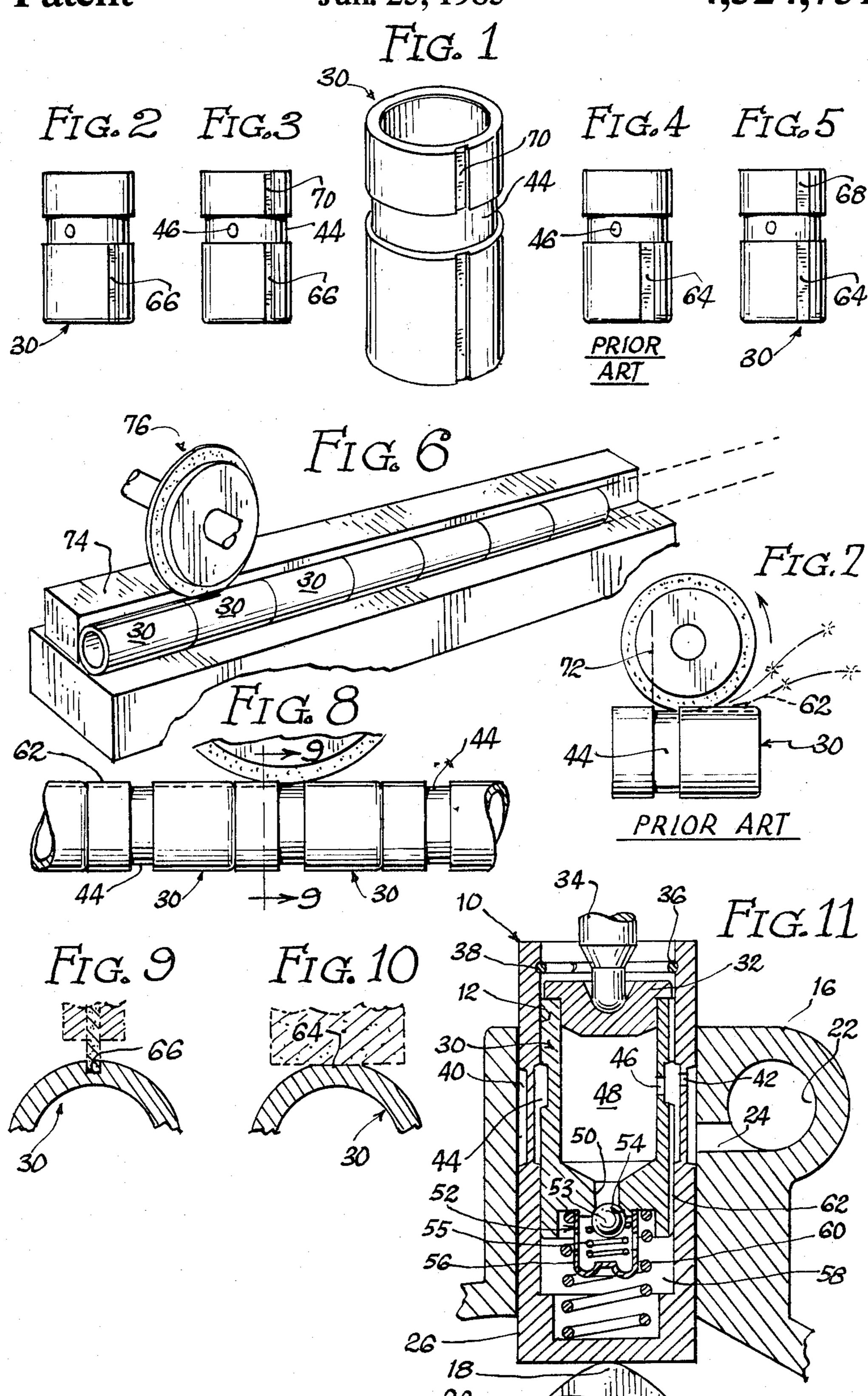
HYDRAULIC VALVE LIFTER WITH CONTINUOUS VOID
