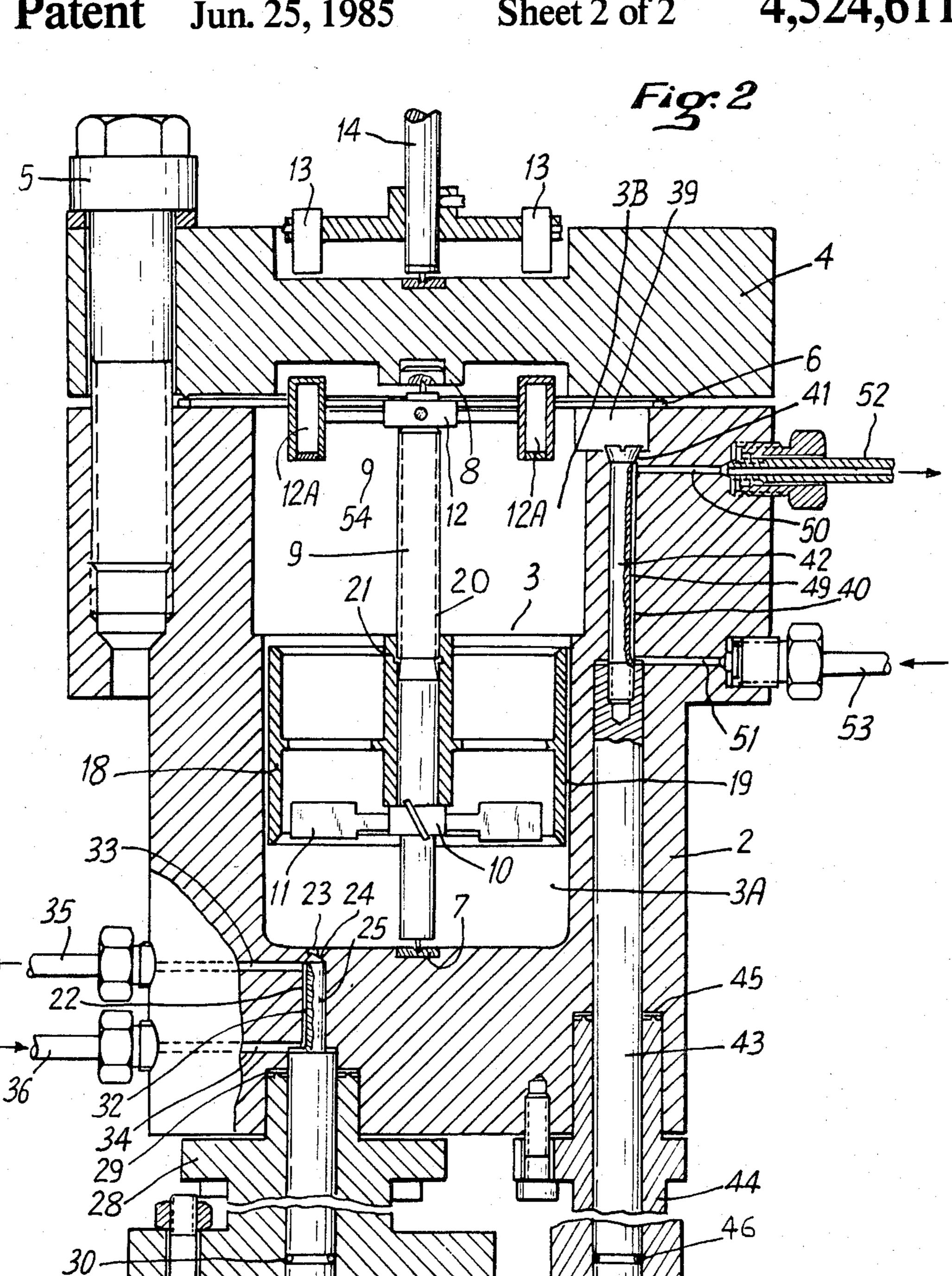
RHEOMETER FOR MEASURING HIGH PRESSURE AND HIGH TEMPERATURE WITH SAMPLING
