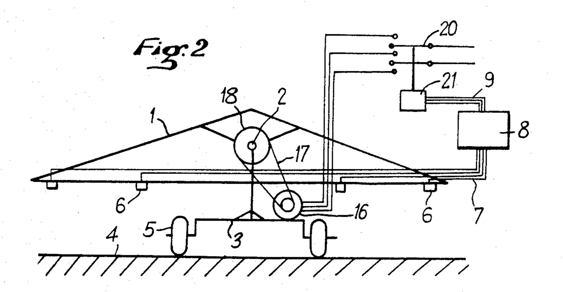
PROCESS FOR THE STABILIZATION WITH RESPECT TO A DESIRED PATH OF A MEMBER WHICH IS MOVABLY MOUNTED ACCORDING TO AT LEAST ONE COMPONENT OF MOVEMENT AND ITS APPLICATION TO THE STABILIZATION OF A SPRAY MANIFOLD
