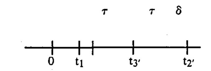
In the above illustration,  $t_{3'}$  is the same as in the preceding diagram since the distance to the target has not changed. However, the measuring light pulse arriving at  $t_{3'}$  at the receiver is the first of the two pulses to arrive and is used to initiate the start signal for the time measurement.
