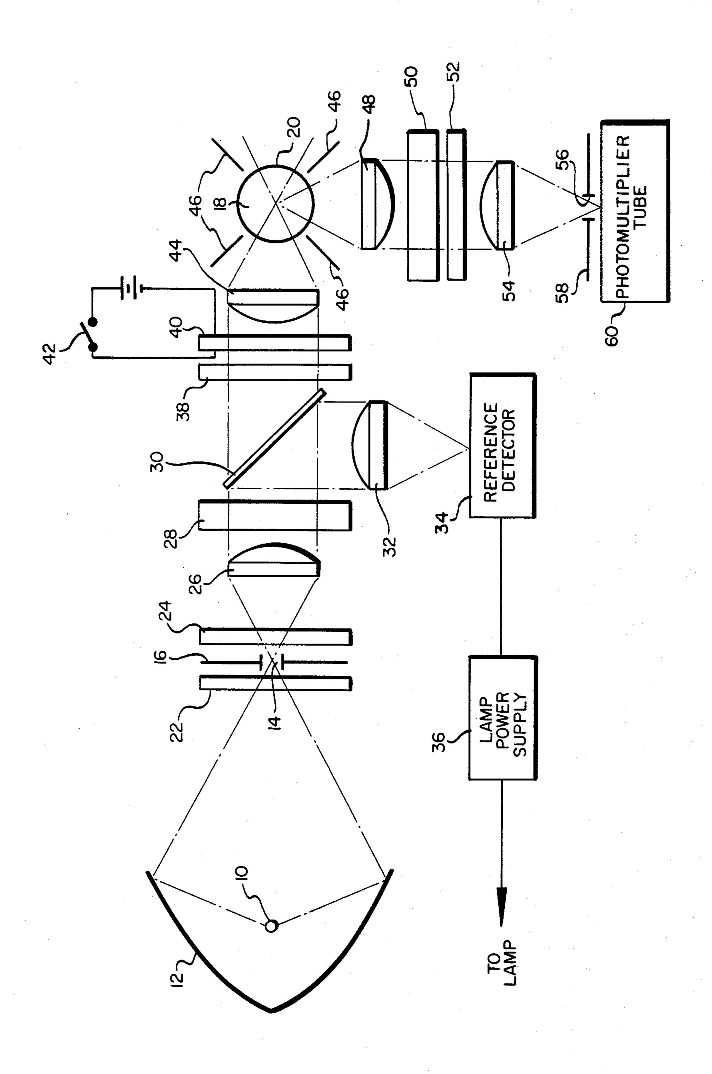
OPTICAL APPARATUS FOR FLUORESCENCE POLARIZATION INSTRUMENT
