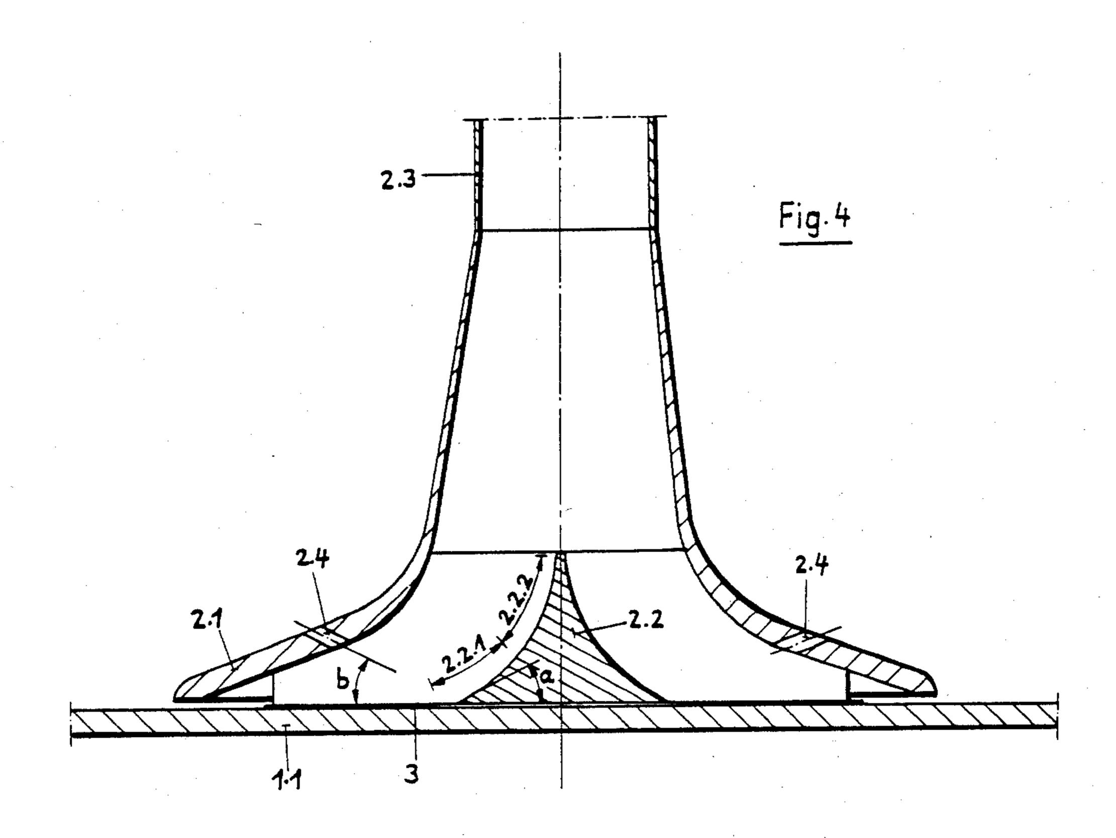
ROTARY DRYER WITH ROTARY LOW-PRESSURE SYPHON
