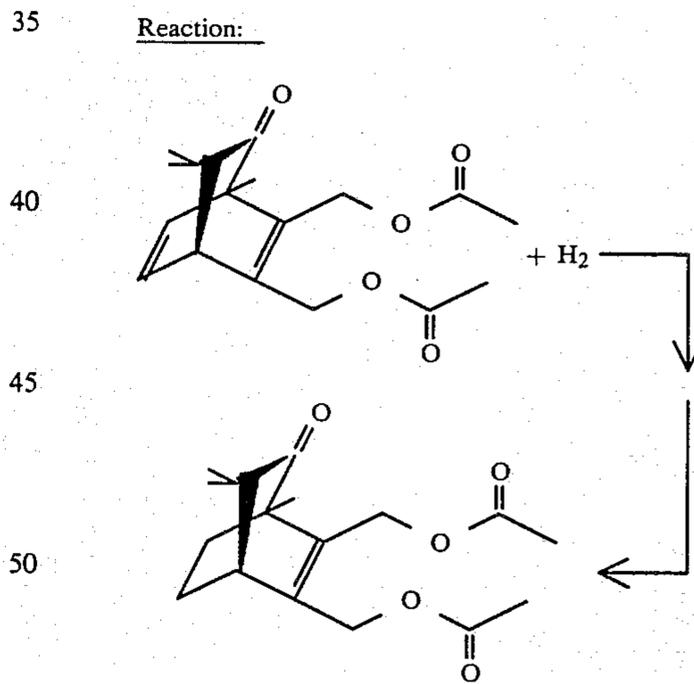
To a 450 ml Parr mini-pressure reactor is charged 15 grams of 5,6-bis(hydroxymethyl)-1,3,3-trimethylbicyclo[2.2.2]octa-5-dien-2-one diacetate produced according to Example IV, 60 ml of isopropyl alcohol and 0.3 grams of 10% palladium-on-carbon.
