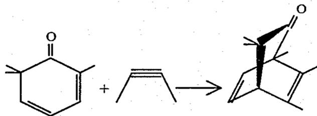
Into a 450 ml Parr mini-pressure reactor is placed 25 grams of 2,6,6-trimethylcyclohexa-2,4-dien-1-one dimer, 75 ml of toluene and 12.4 grams of 2-butyne.
