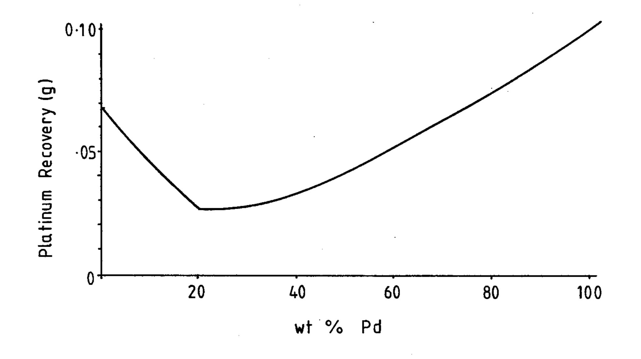
Variation of collection efficiency with gold content of Pd-Au alloys.
