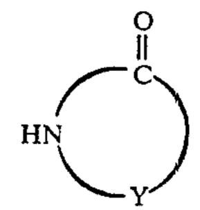
wherein Y is an alkylene group having from 3 to 12 carbon atoms, in particulate form, and an organomagnesium-containing material. The process is carried out at a temperature below the melting point of the lactam monomer but at a temperature sufficient to convert at least a portion of the lactam monomer to said lactam-magnesium compound in pulverulent form. The lactam-magnesium compound is useful as a catalyst for anionic lactam polymerization.
