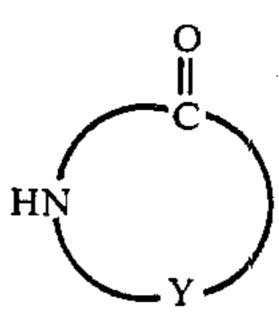
wherein Y is an alkylene group having from 3 to 12 carbon atoms, in particulate form, into intimate admixture with the organomagnesium-containing material at a temperature below the melting point of the lactam monomer but at a temperature sufficient to convert at least a portion of the lactam monomer to said lactam-magnesium compound in pulverulent form.
