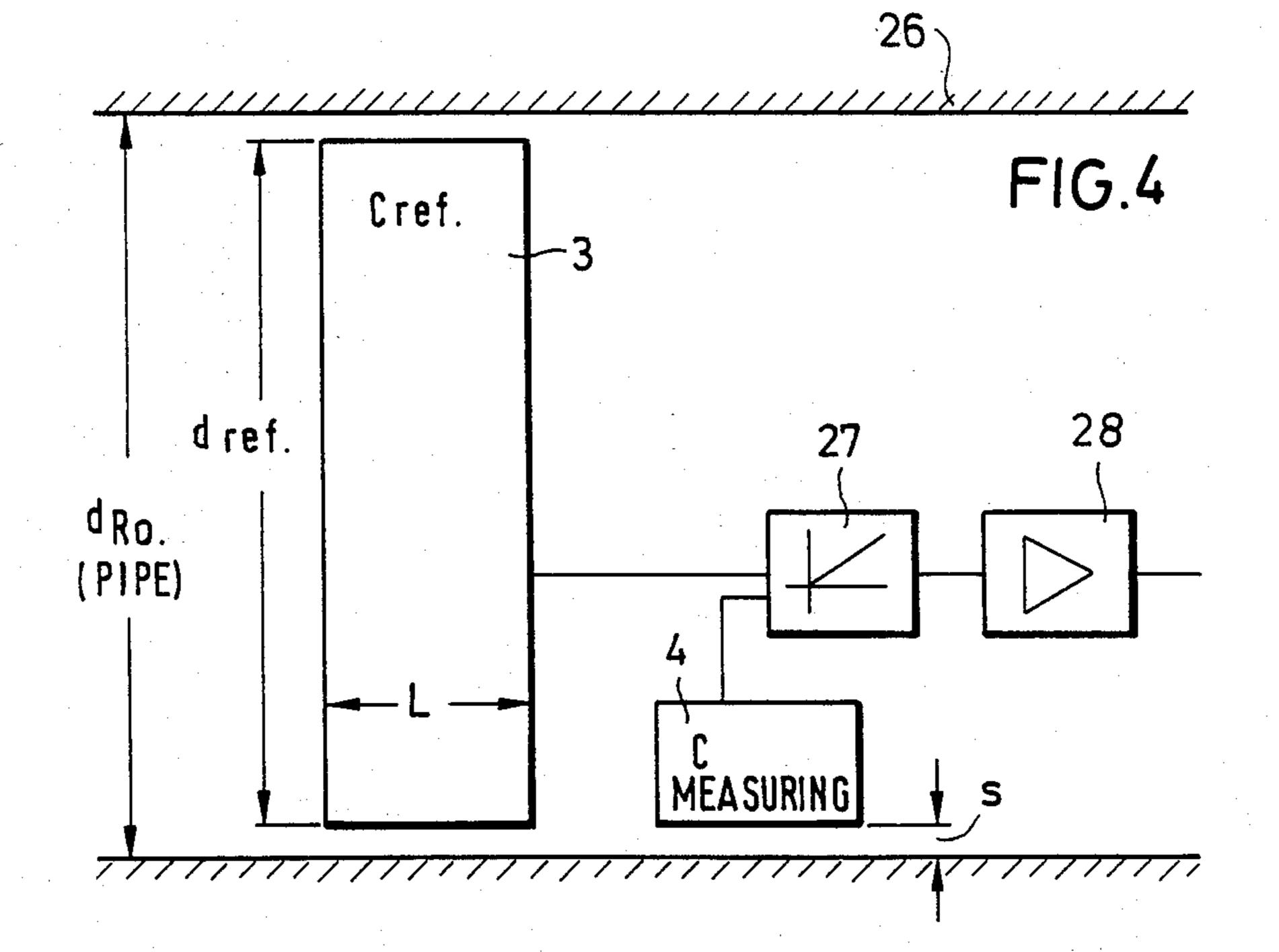
METHOD AND ARRANGEMENT USING A PAIR OF RESONANT CIRCUITS FOR DETERMINING AND INDICATING THE POSITION OF AN UNEVENESS IN THE INNER SURFACE OF PIPES OR OTHER TYPES OF CYLINDRICAL STRUCTURES
