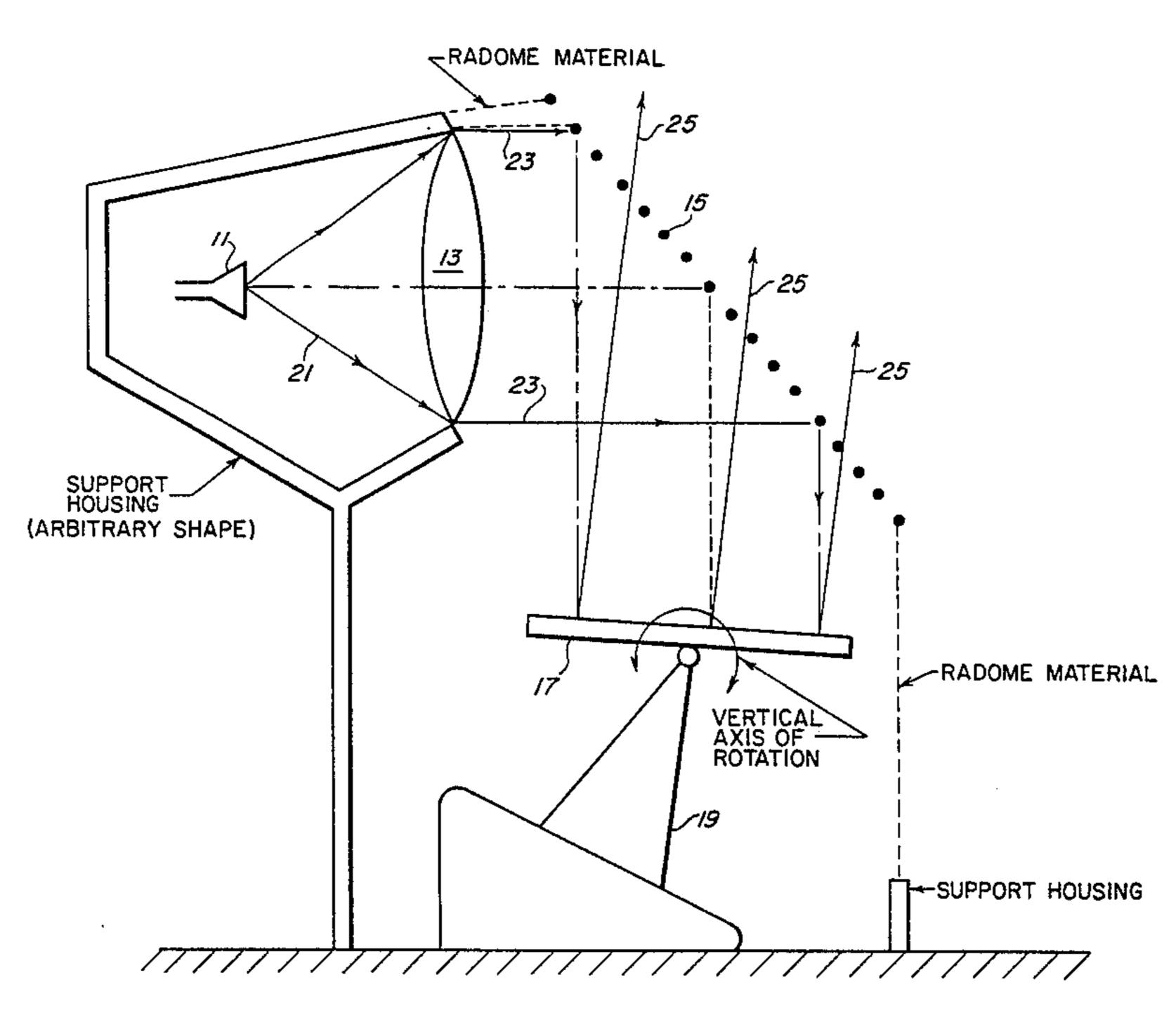
INDIRECT FEED FOR THE TWO-AXIS MIRROR ANTENNA (ONLY ONE AXIS ILLUSTRATED)
