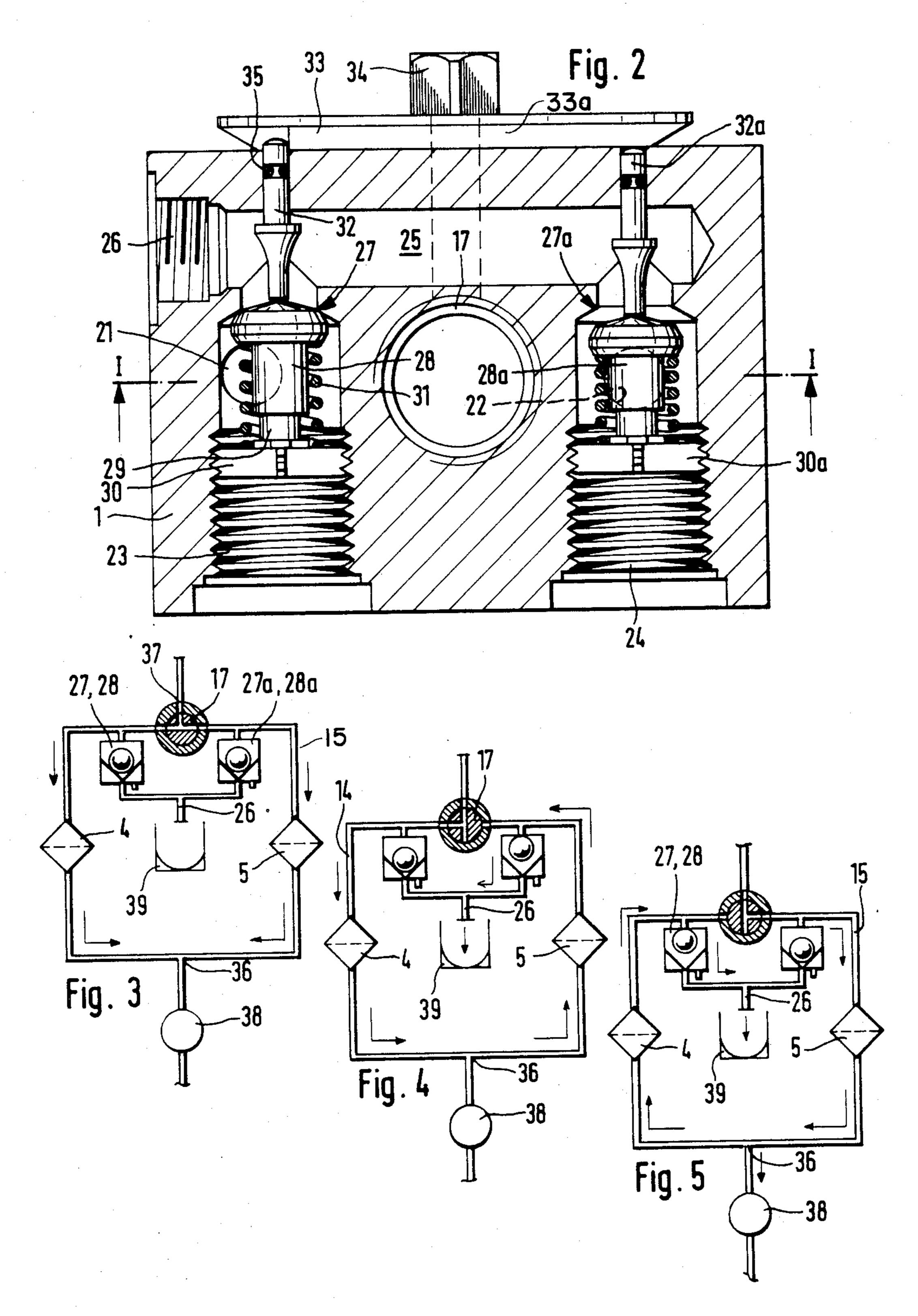
FIGS. 3, 4 and 5 are schematic fluid flow diagrams showing three possible operating conditions of the apparatus of FIGS. 1 and 2.
