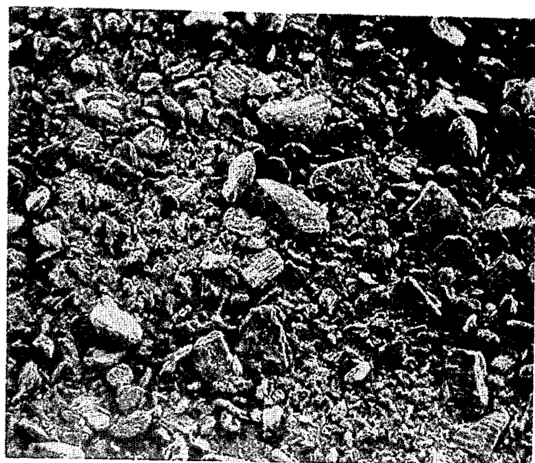
DRY MILLED CORN BRAN MODIFIED AFTER EXTRUSION AND MILLING.
