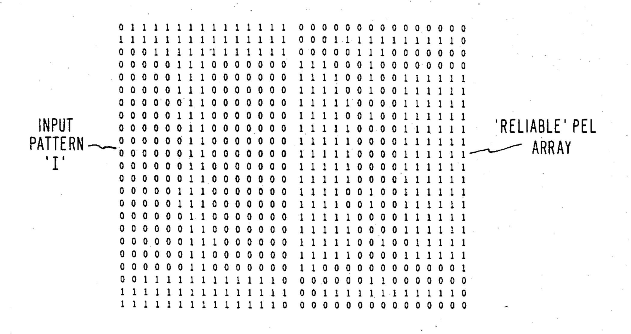
A BIT REPRESENTATION OF AN INPUT PATTERN AND ITS RELIABLE PEL ARRAY FIG.2
