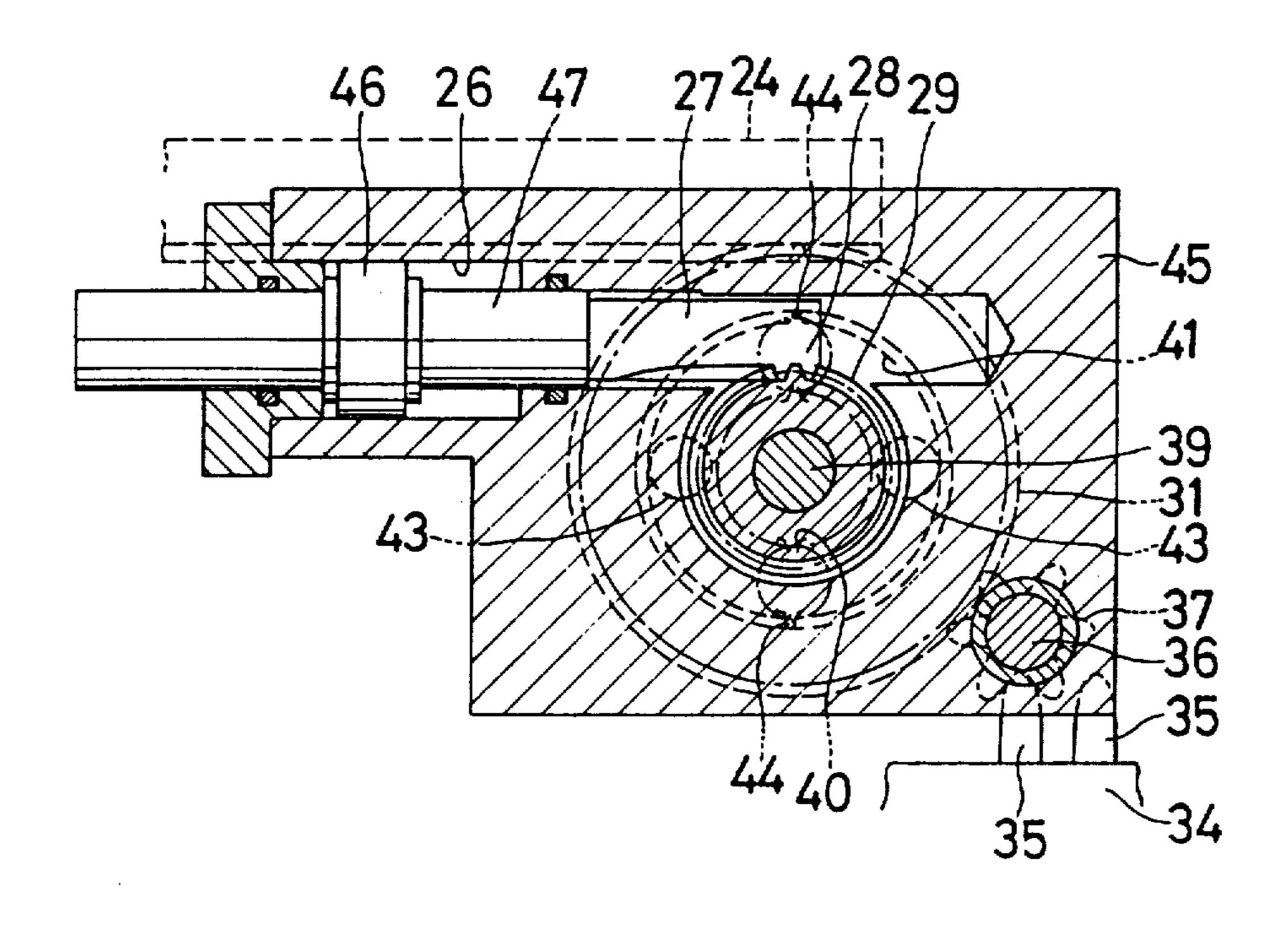
that phase in meshing of the rack and the gear of the star gear shaft will be changed when the rack is recoupled with the star gear shaft, resulting in a problem similar to that experienced in the former case where the star gear shaft is not locked.
