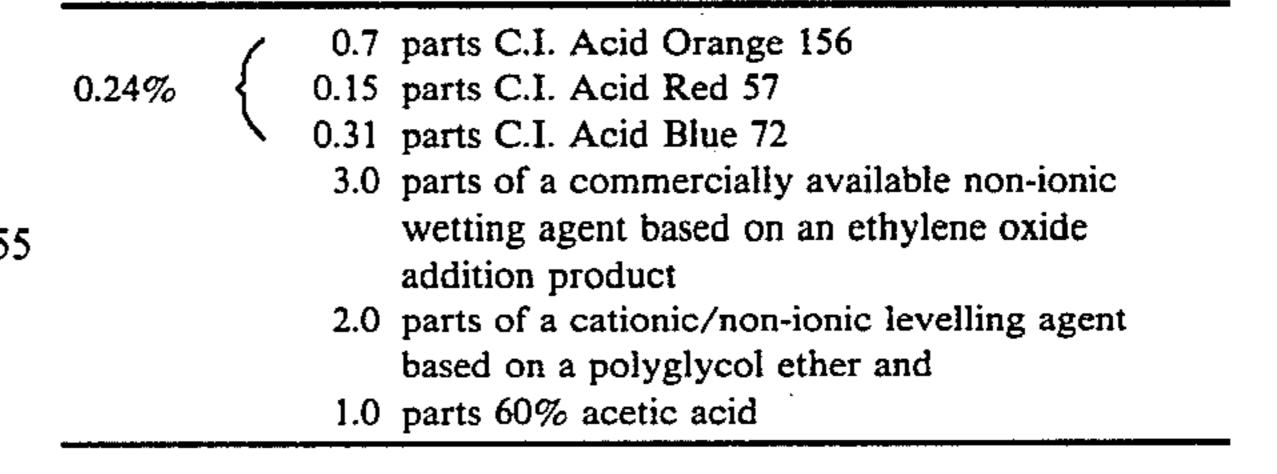
is poured on a loop pile carpet of polyamide 6.6 fibre group 3 having a synthetic backing. The liquor absorption amounts to 210% based on the weight of the carpet.
