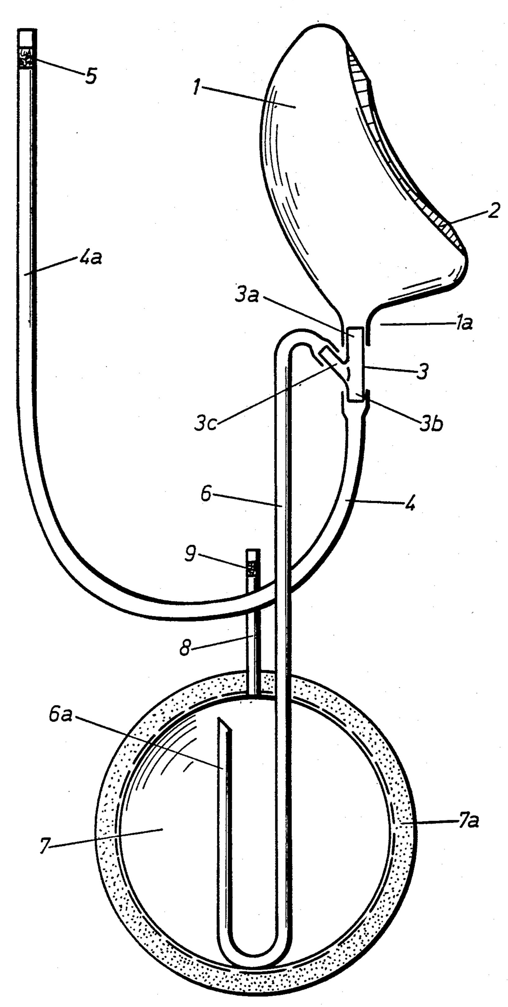
APPARATUS FOR SEPARATELY CATCHING SUCCESSIVE STREAMS OF URINE AT TAKING SAMPLES TO LABORATORIAL AND BACTERIOLOGICAL EXAMINATION
