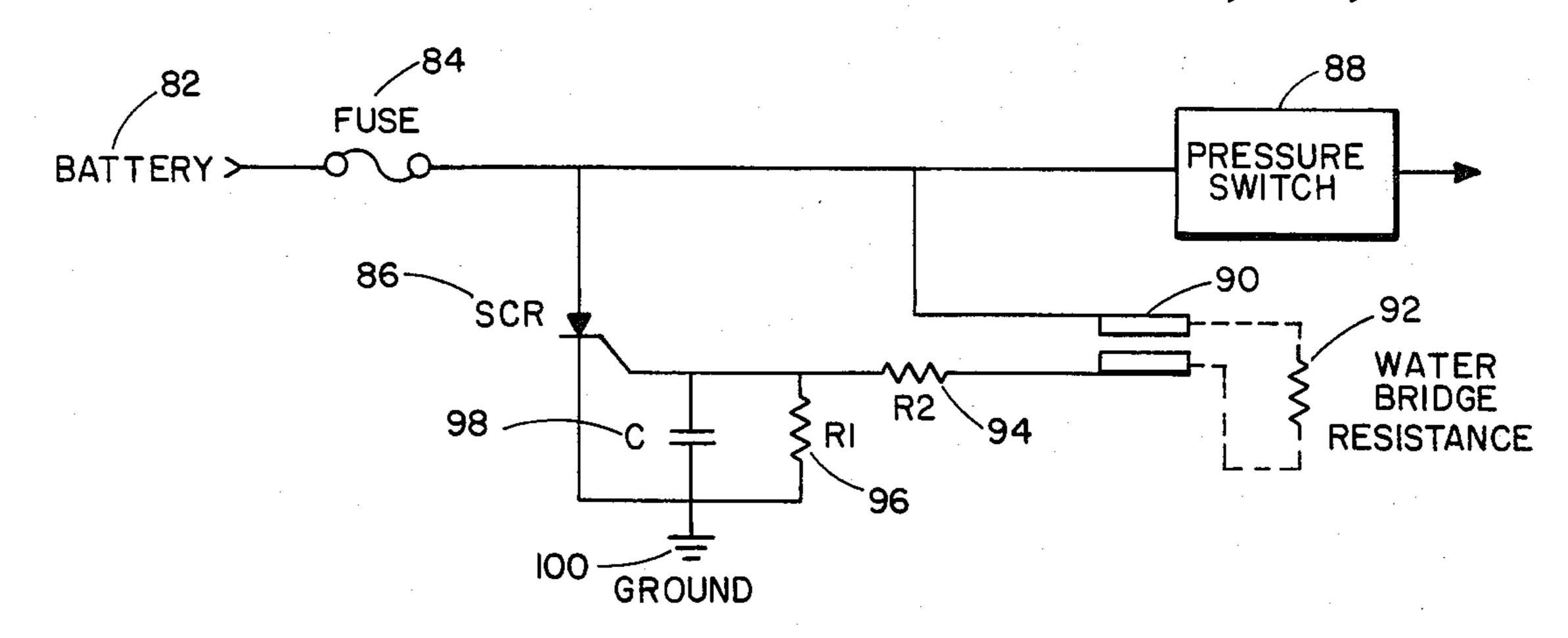
FIG. 4. WATER INTRUSION FAIL-SAFE CIRCUIT.
