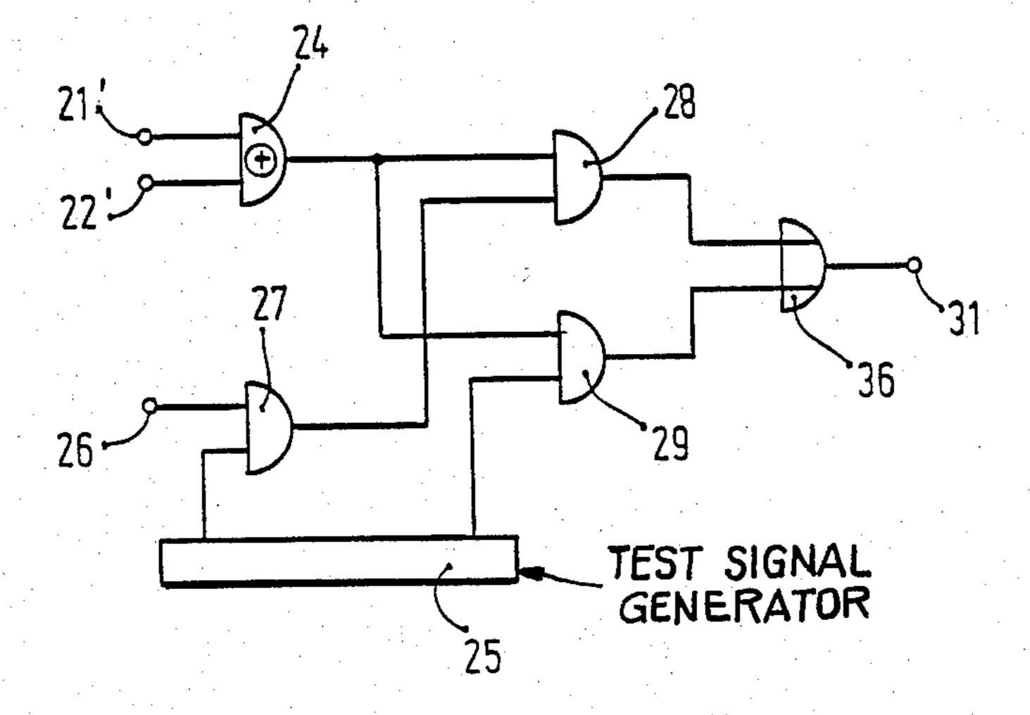
a warning to an operator of the motor vehicle that the circuits are not functioning properly, which output signal can additionally be used to disable the anti-brake lock circuit, or to carry out other switching functions.
