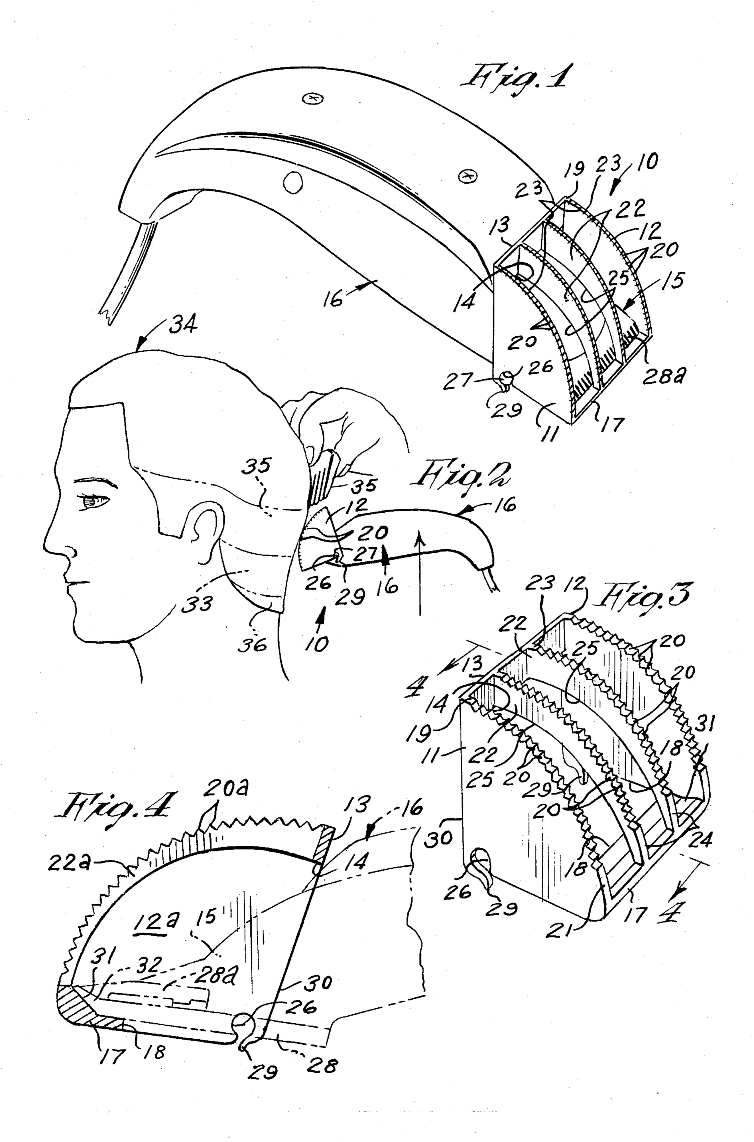
This invention relates to hair cutting instruments, and more particularly, to a taper gauge device for hair clip- 5 pers.
