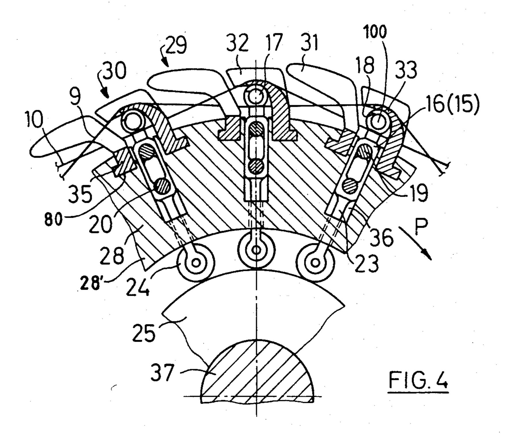
APPARATUS FOR GUIDING A FLUID MEDIUM DRIVEN WEFT THREAD IN THE SHED OF A WEAVING MACHINE AND USE OF THE APPARATUS AT A MULTIPLE LONGITUDINAL TRAVERSING SHED WEAVING MACHINE
