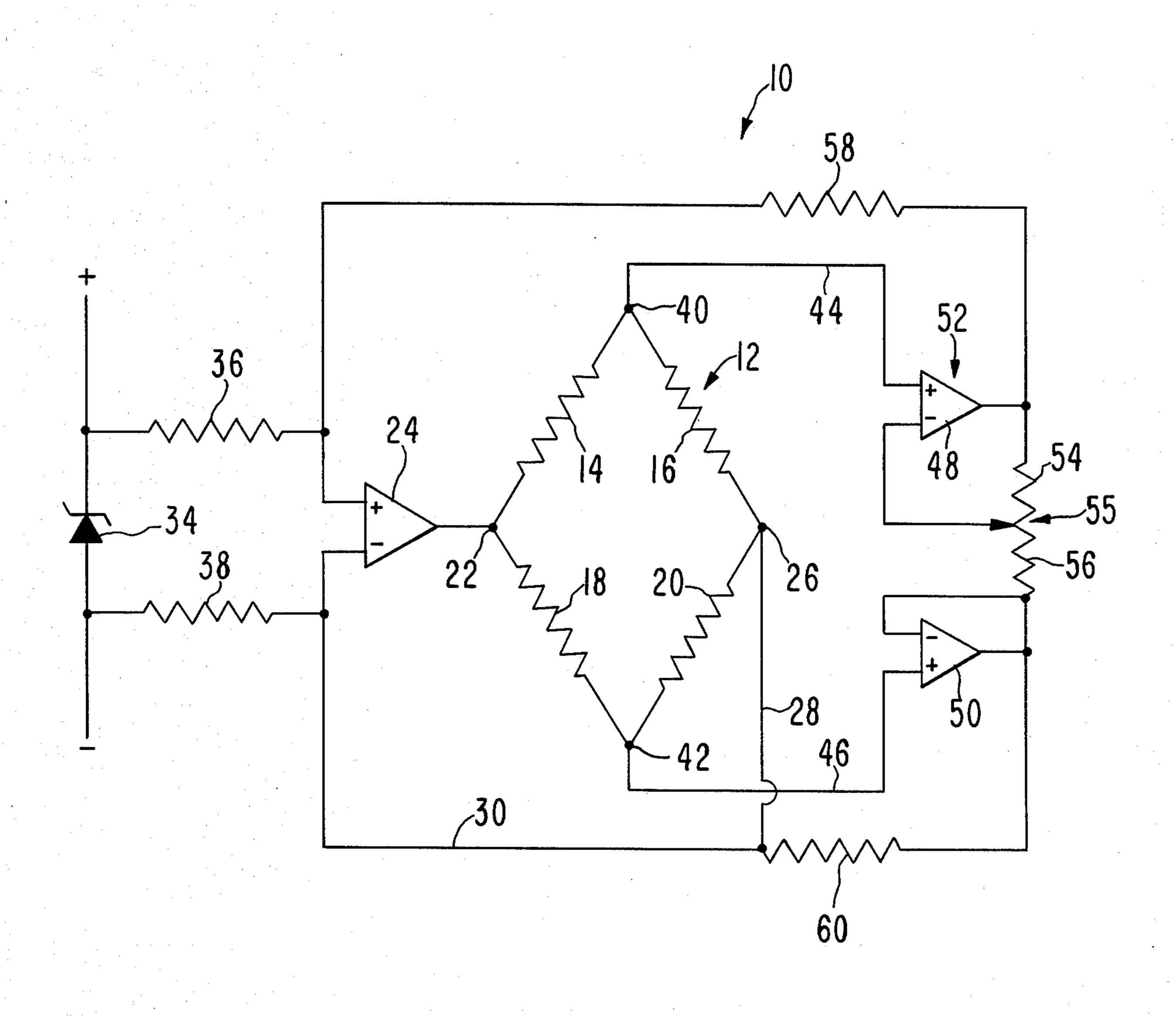
CIRCUIT FOR LINEARIZATION OF TRANSDUCER
