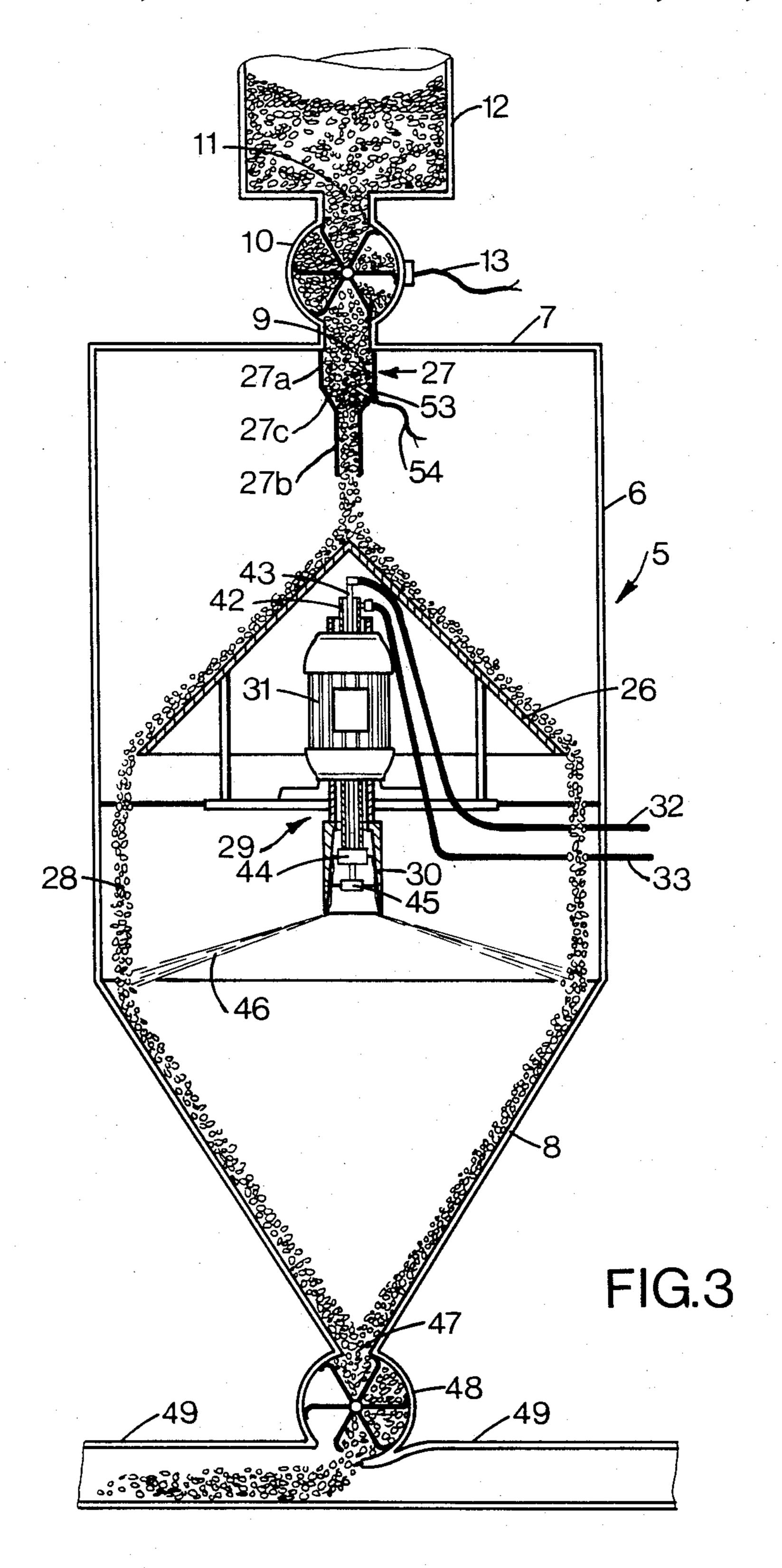
METHOD FOR APPLYING A SCREED COAT TO A ROOF SURFACE
