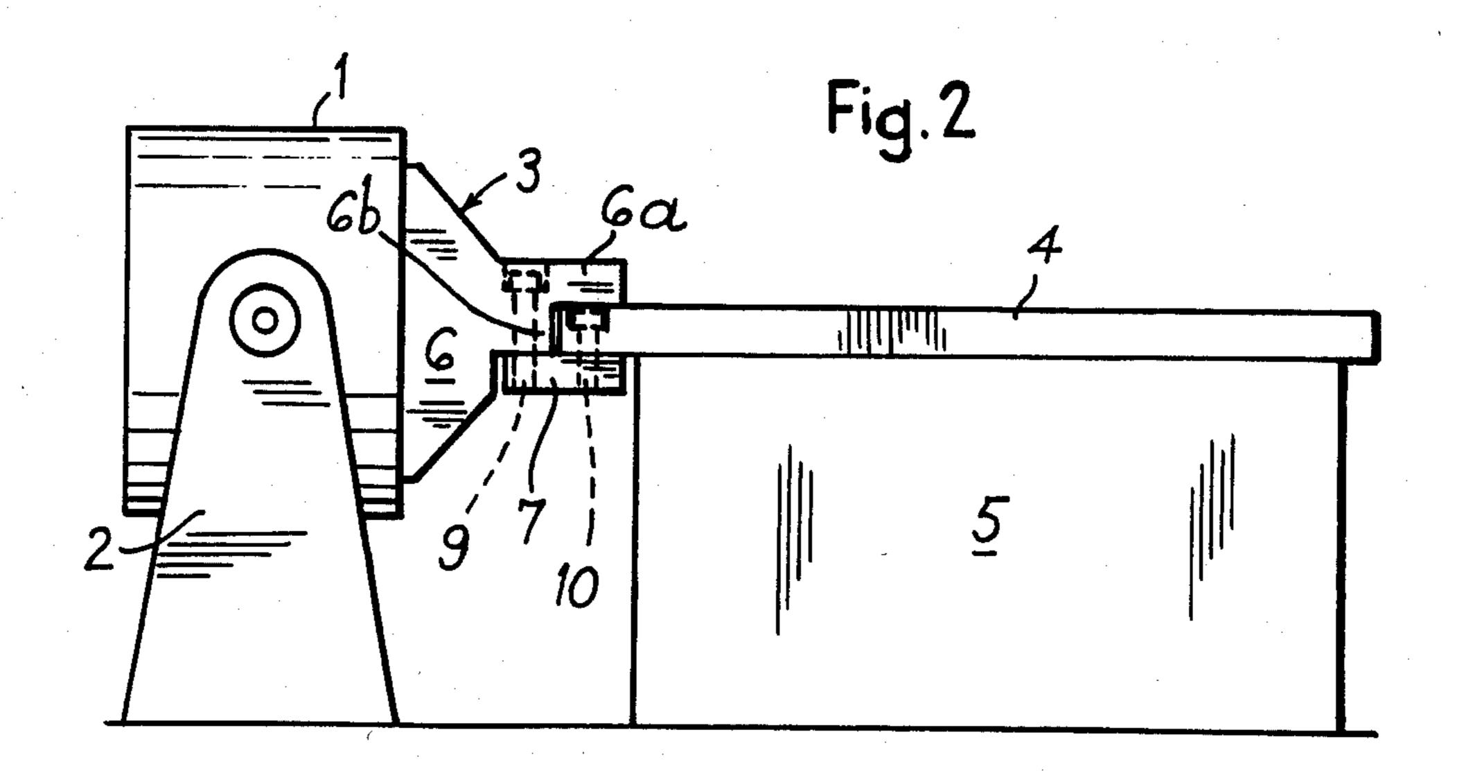
The present invention relates to vibration testing apparatus, otherwise known as shakers, such as are 5 employed in industry for the vibration testing of industrial elements and components.
