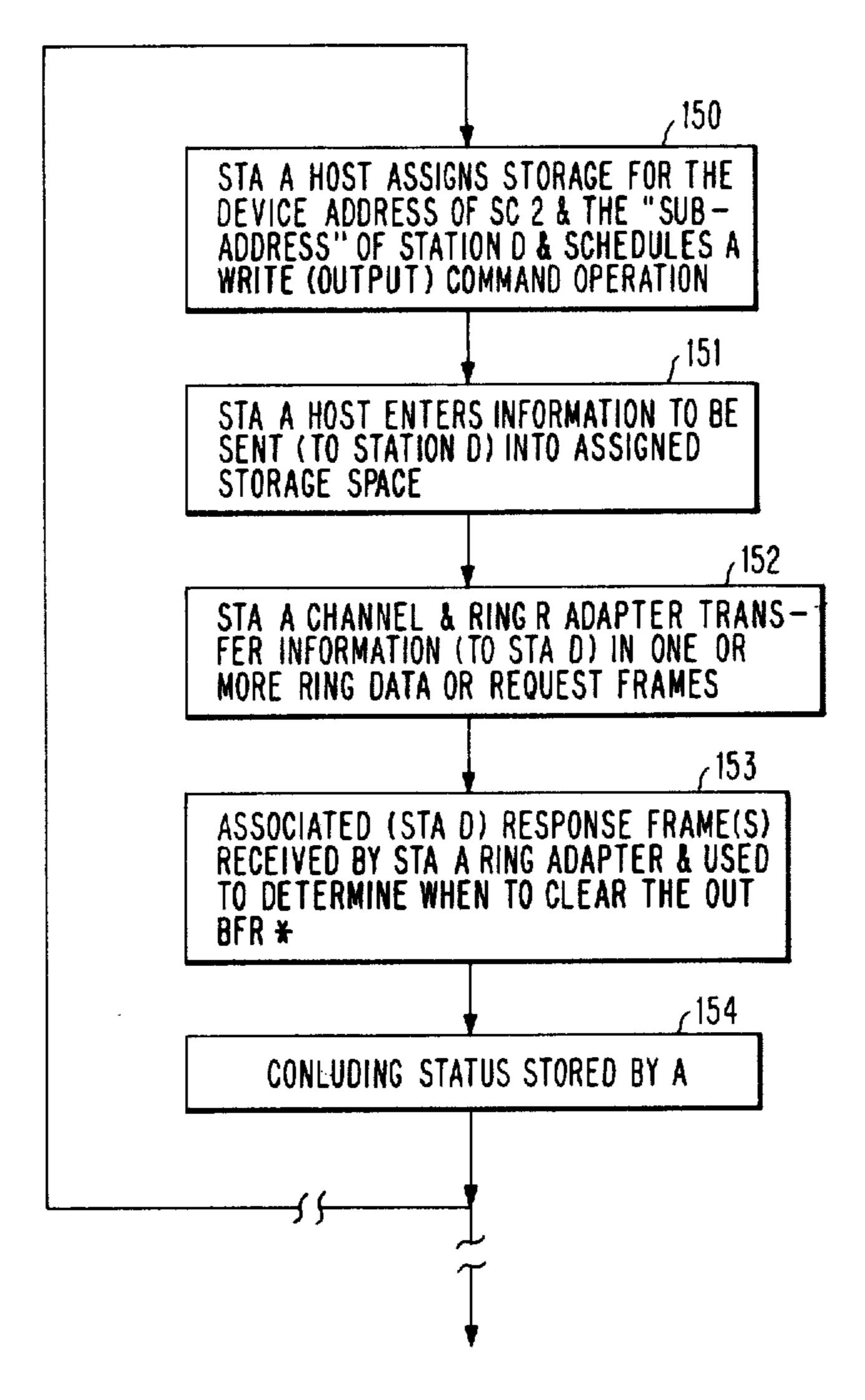
\* — IF MORE THAN ONE FRAME IS BEING SENT, THE OUT BUFFER IS CLEARED WITH EACH POSITIVE ACKNOWLEDGEMENT (FROM D) & SIGNAL IS GIVEN TO THE CHANNEL TO "RELOAD" THE BUFFER
