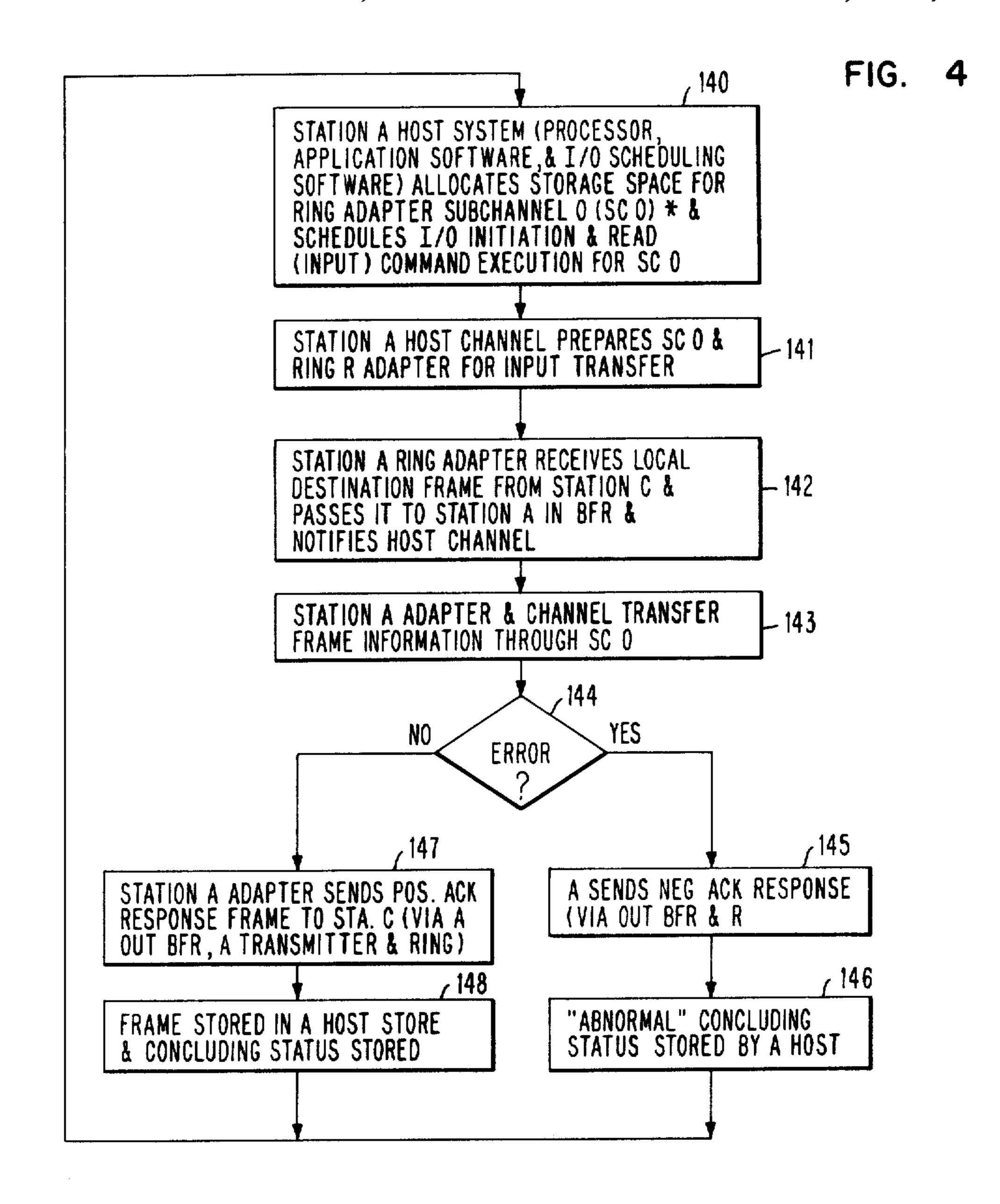
\*-STATION A'S RING ADAPTER HAS A DEVICE ADDRESS "PERMANENTLY ASSOCIATED" WITH SC 0
