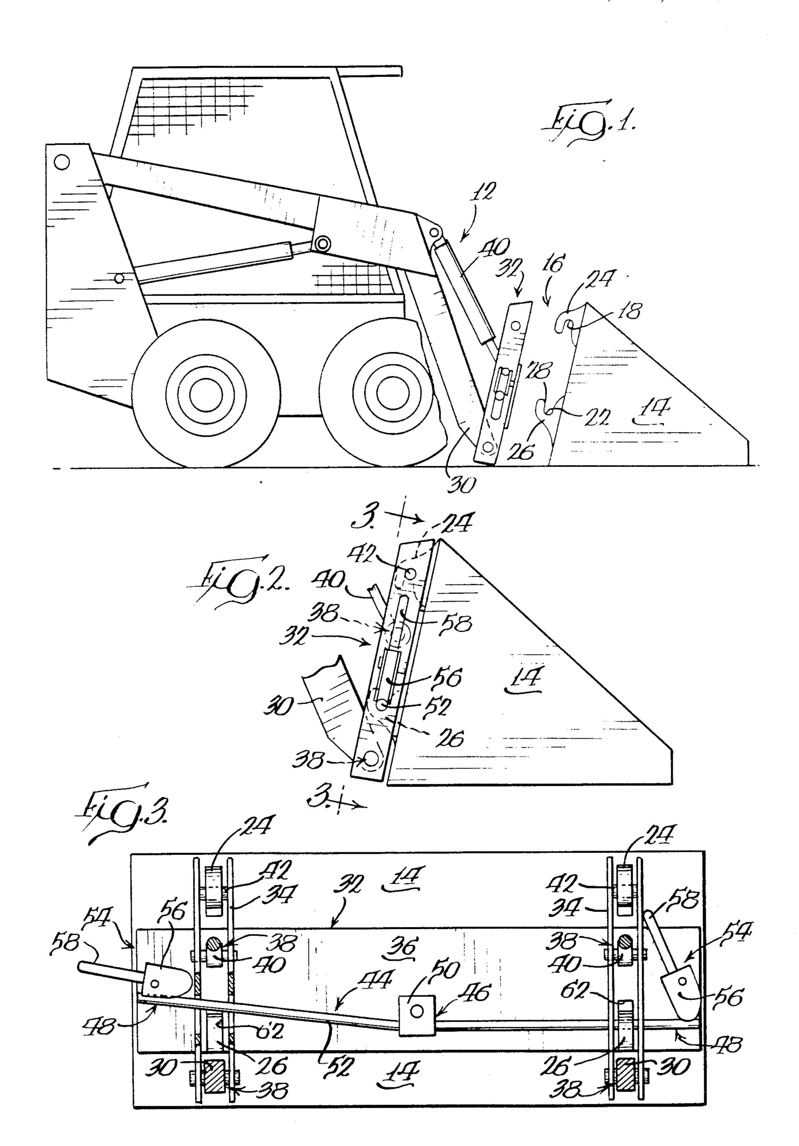
by the first recess and the second latching means engages the second recess to attach the implement on the frame member.
