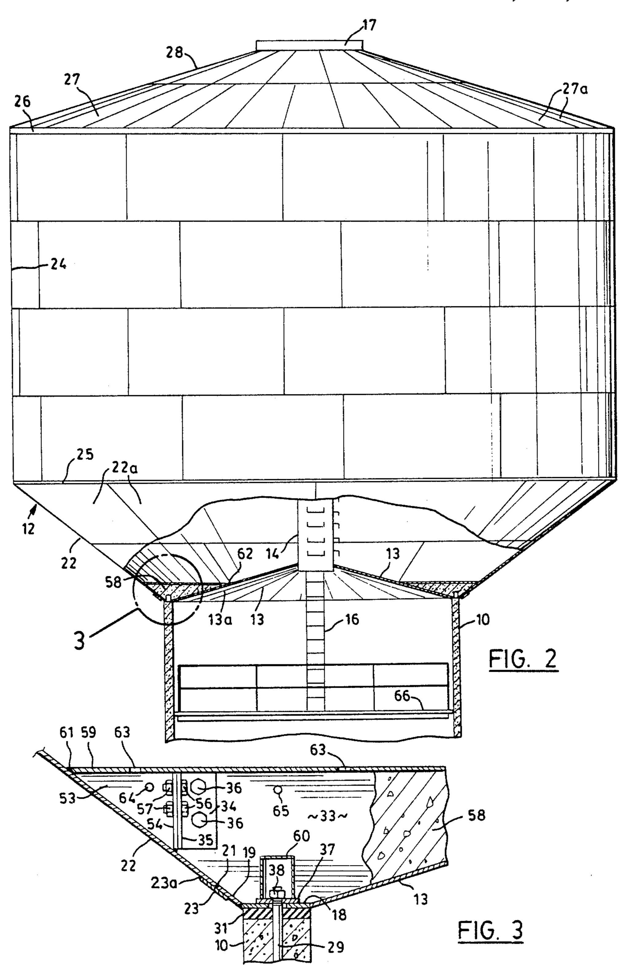
FIG. 2 shows a side view, partly in vertical section, of the upper end of the tank;
