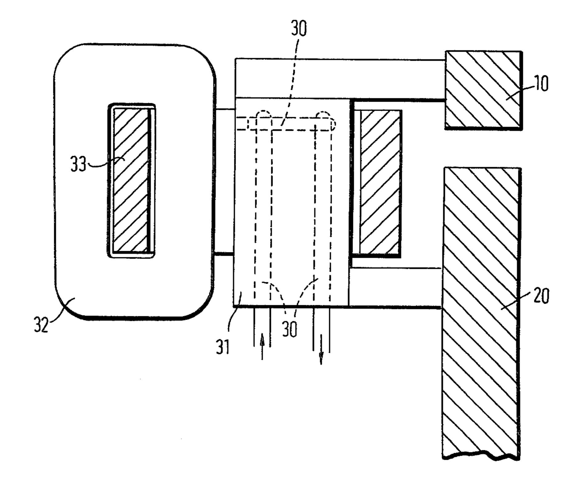
example copper, in the form of closed loops. High currents are induced in these loops by means of energising coils which may either be wound about the conductor, or may be coupled thereto by ferromagnetic cores.
