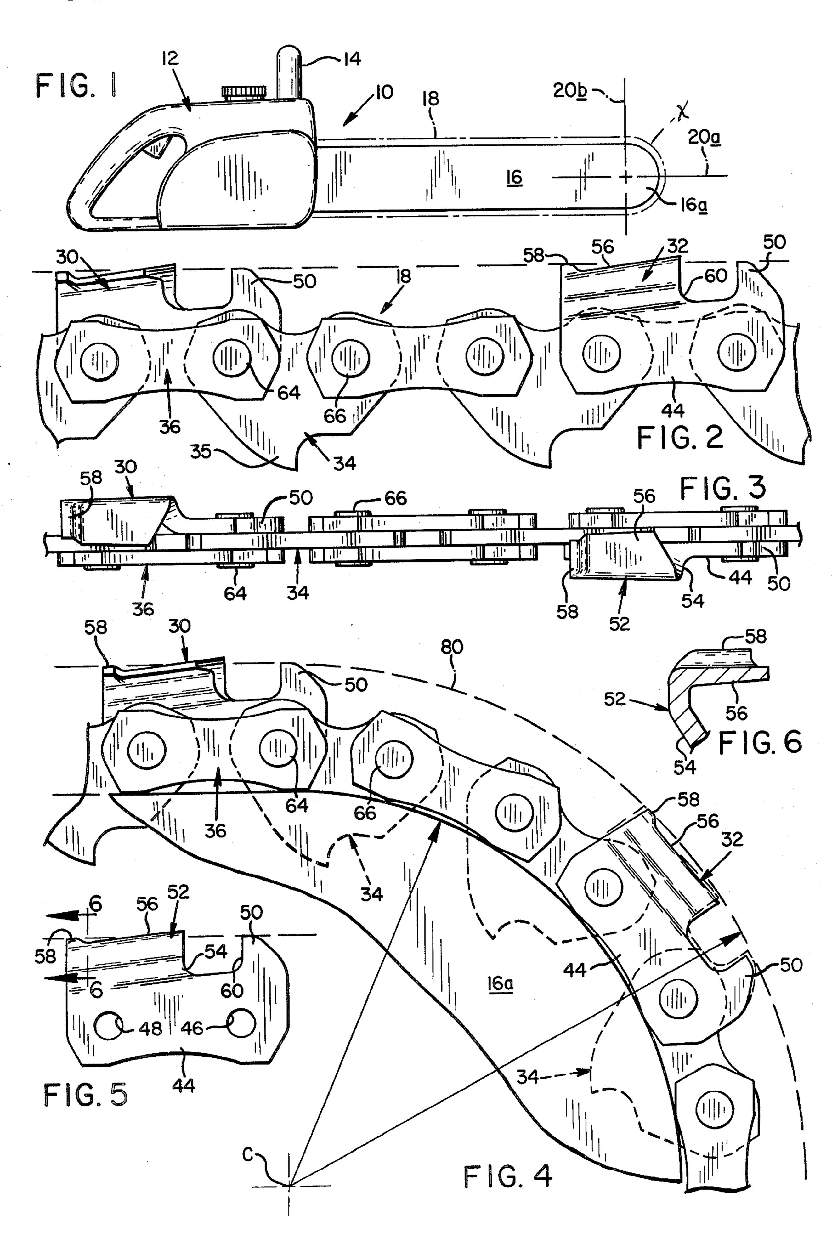
FIG. 4 illustrates the nose portion of a chain saw bar
