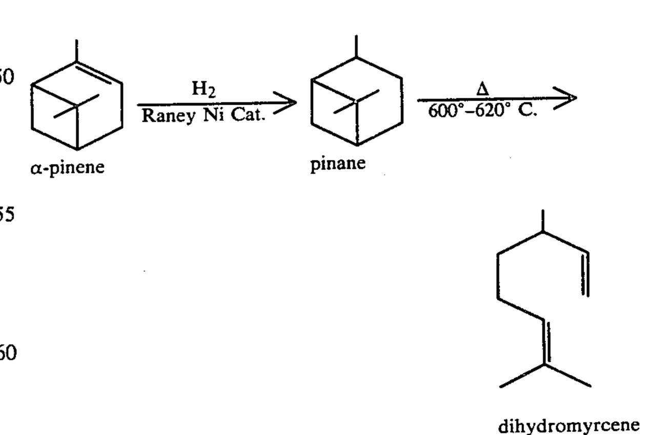
We prefer to effect hydrogenation with molecular hydrogen under superatmospheric pressure, e.g., 70 to 80 psig. in the liquid phase and in the presence of a solid contact catalyst, e.g., Raney nickel until 1 mole of hy-
