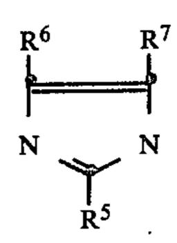
where R<sup>5</sup>, R<sup>6</sup> and R<sup>7</sup> have the above meanings, is reacted with NaOCH<sub>3</sub>, in a solvent, eg. dimethylformamide, at from 100° to 150° C. in the course of from 1 to 20 hours, the CH<sub>3</sub>OH is distilled off, the product thus obtained is reacted with a compound of the formula R<sup>4</sup>-Cl where R<sup>4</sup> has the above meanings, the NaCl is separated off from the reaction mixture, and the end product is isolated from the solvent.
