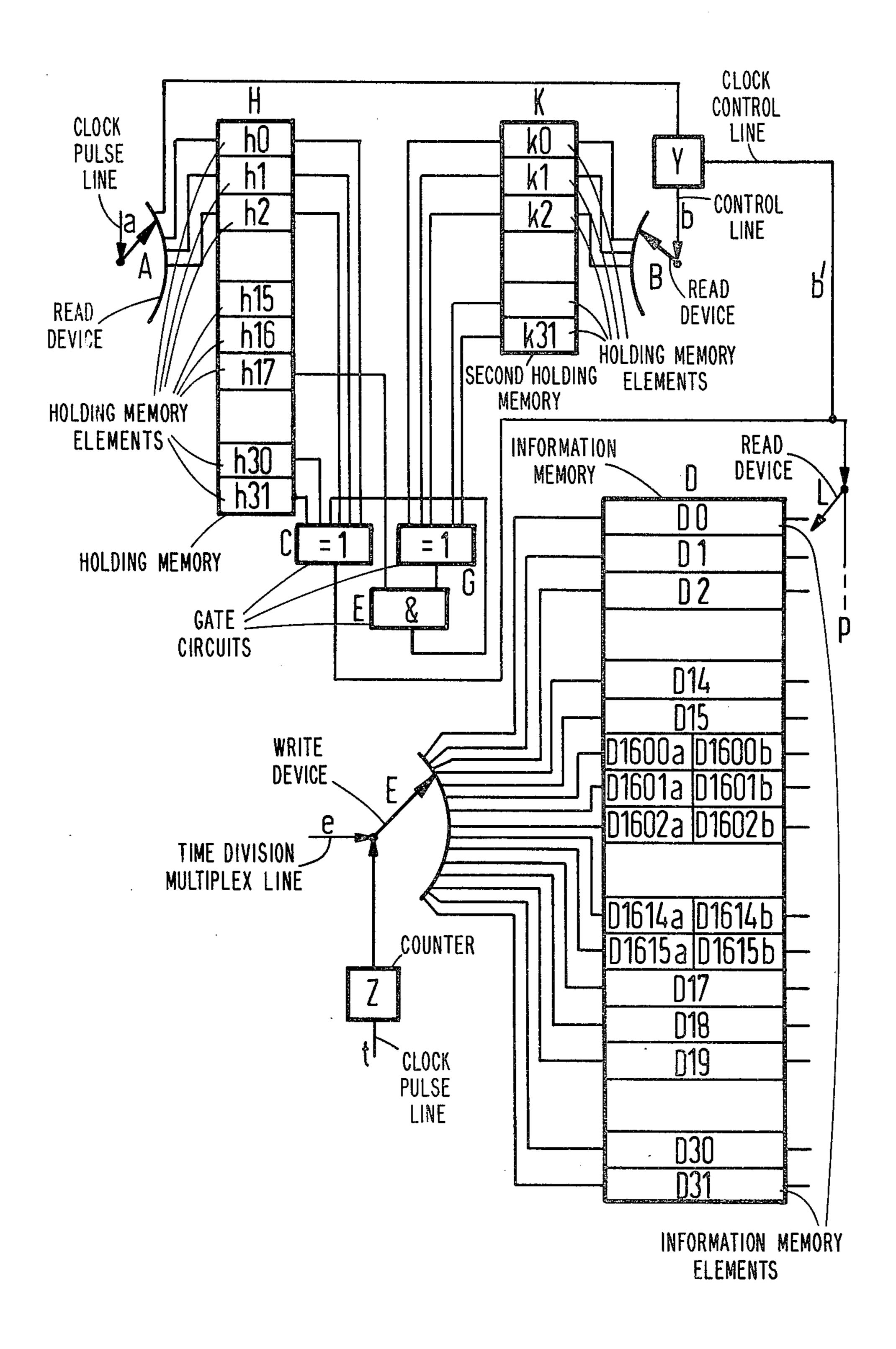
CIRCUIT ARRANGEMENT FOR TIME-DIVISION MULTIPLEX TELECOMMUNICATION EXCHANGE SYSTEMS COMPRISING MULTIPLEX LINES WHOSE TIME CHANNELS SERVE PARTIALLY FOR MESSAGE CONNECTIONS AND PARTIALLY FOR THE TRANSMISSION OF SIGNALING INFORMATION
