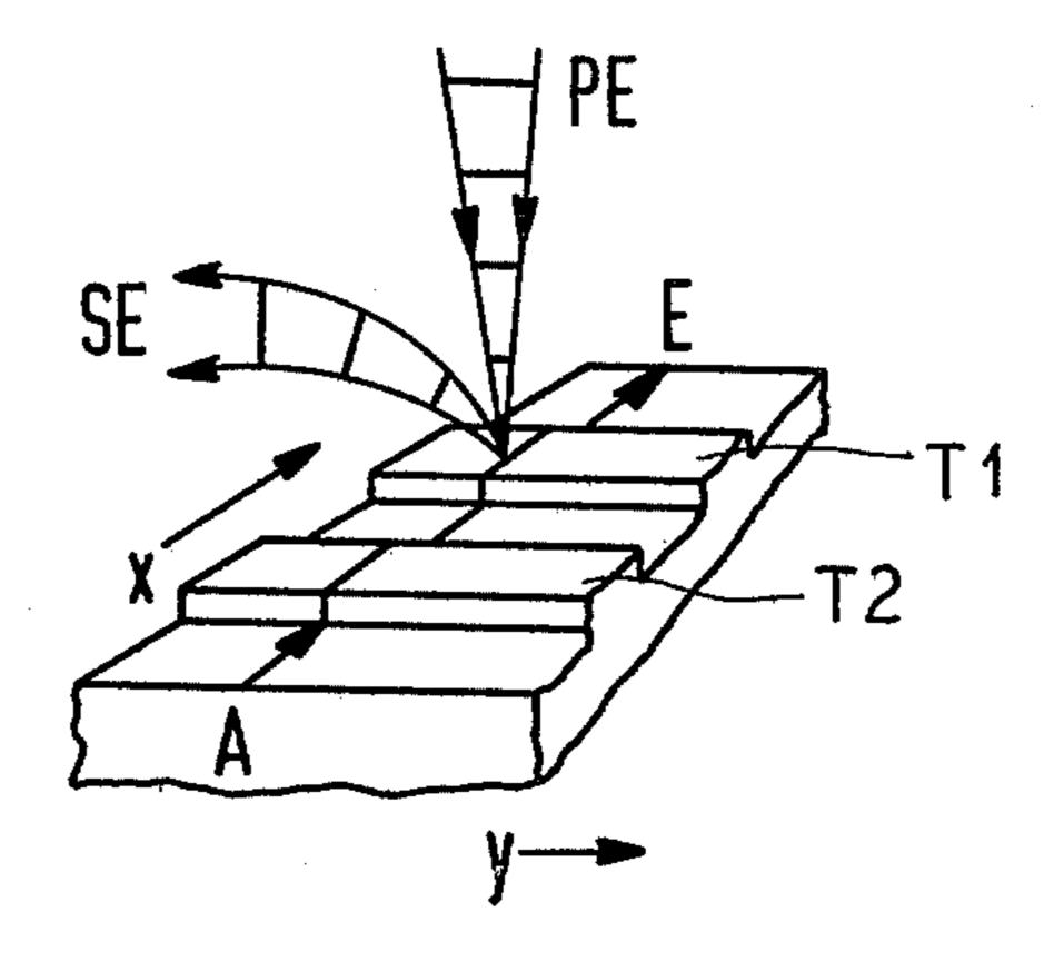
METHOD FOR REPRESENTING LOGICAL STATUS CHANGES OF A PLURALITY OF ADJACENT CIRCUIT NODES IN AN INTEGRATED CIRCUIT IN A LOGIC IMAGE EMPLOYING A PULSED ELECTRON PROBE
